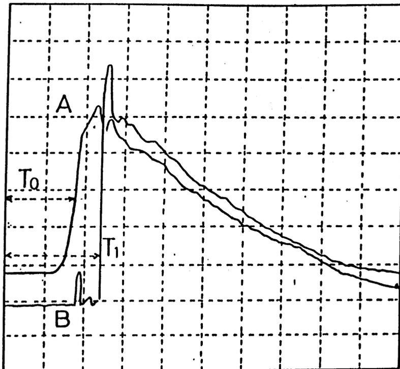
Fig. 8 Impulse voltage and discharge current waveforms
