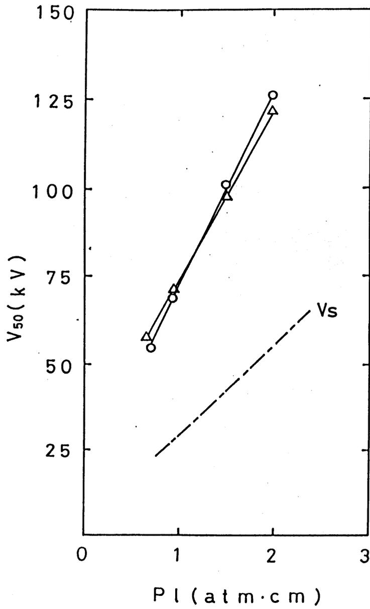
Fig. 4 50% probability of flashover voltage vs  $P l$
