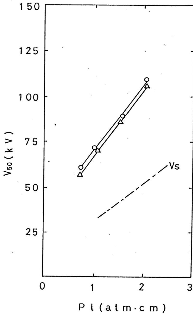
Fig. 7 50% probability of flashover voltage vs  $p l$
