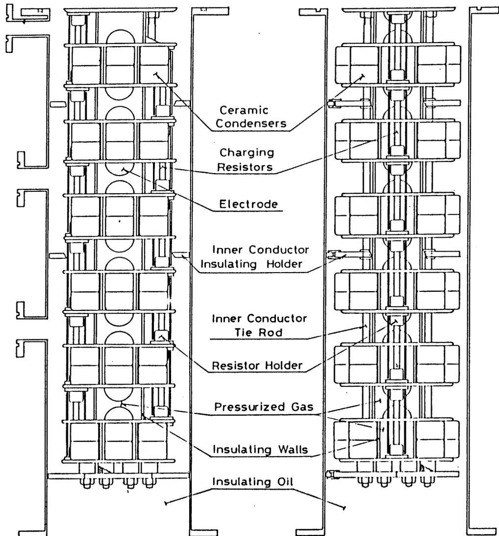
Fig. 1 Layout of the elements in CMG (viewed from two different cross sections)
