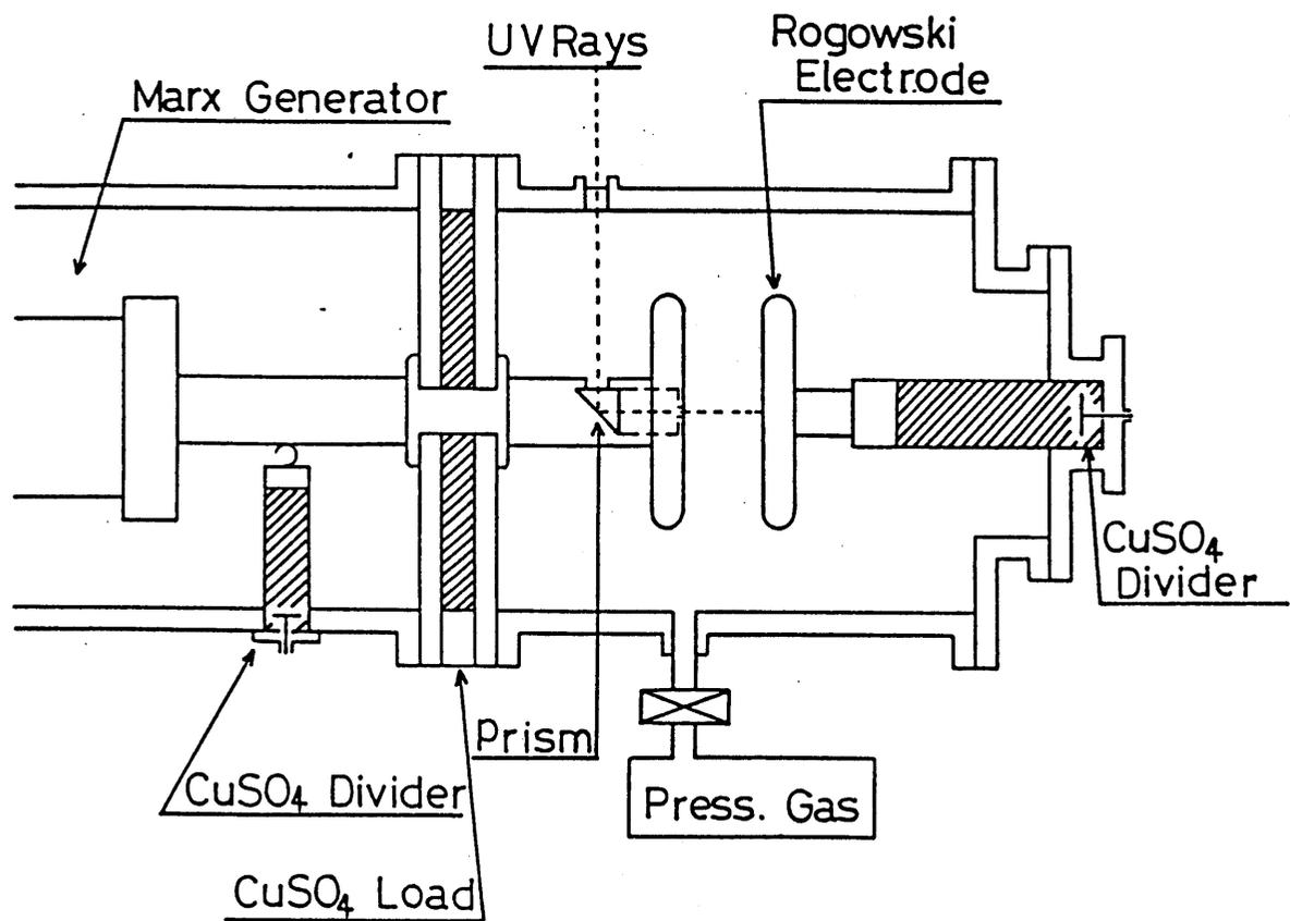
Fig. 2 Test gaps and illumination method of ultraviolet rays
