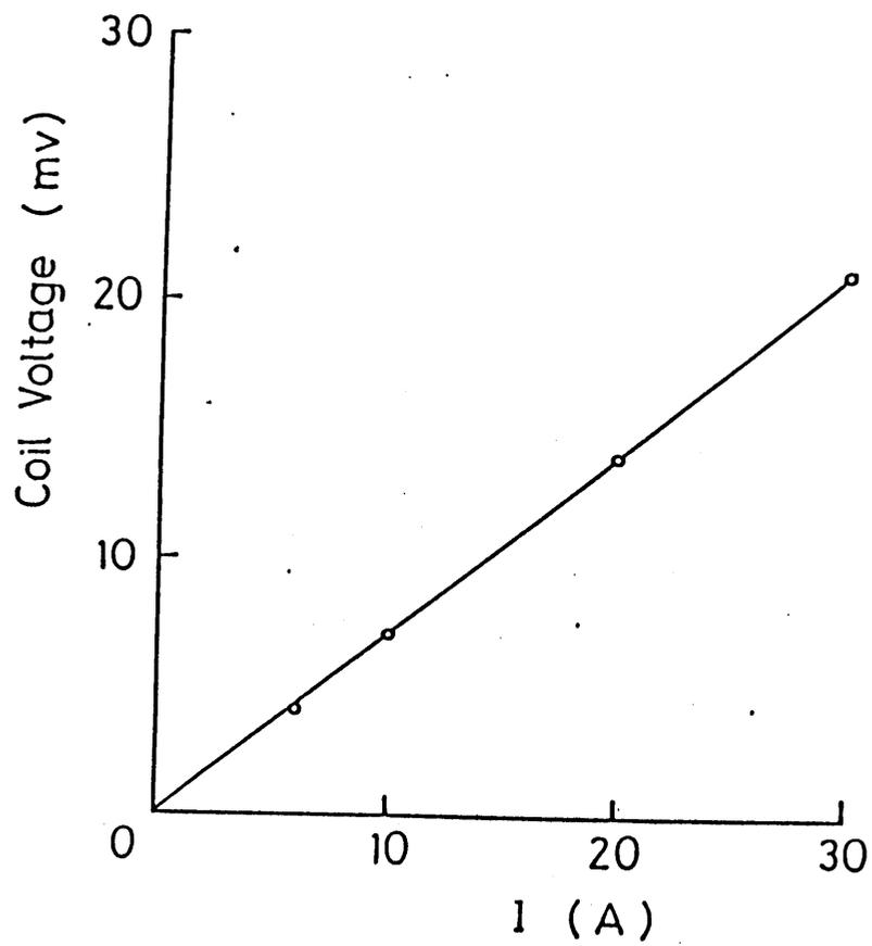
Fig. 12 Voltage vs. current characteristics of pick-up coil
