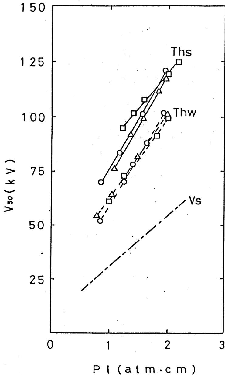
Fig. 6 50% flashover voltage vs  $p l$  characteristics of  $N_2$
