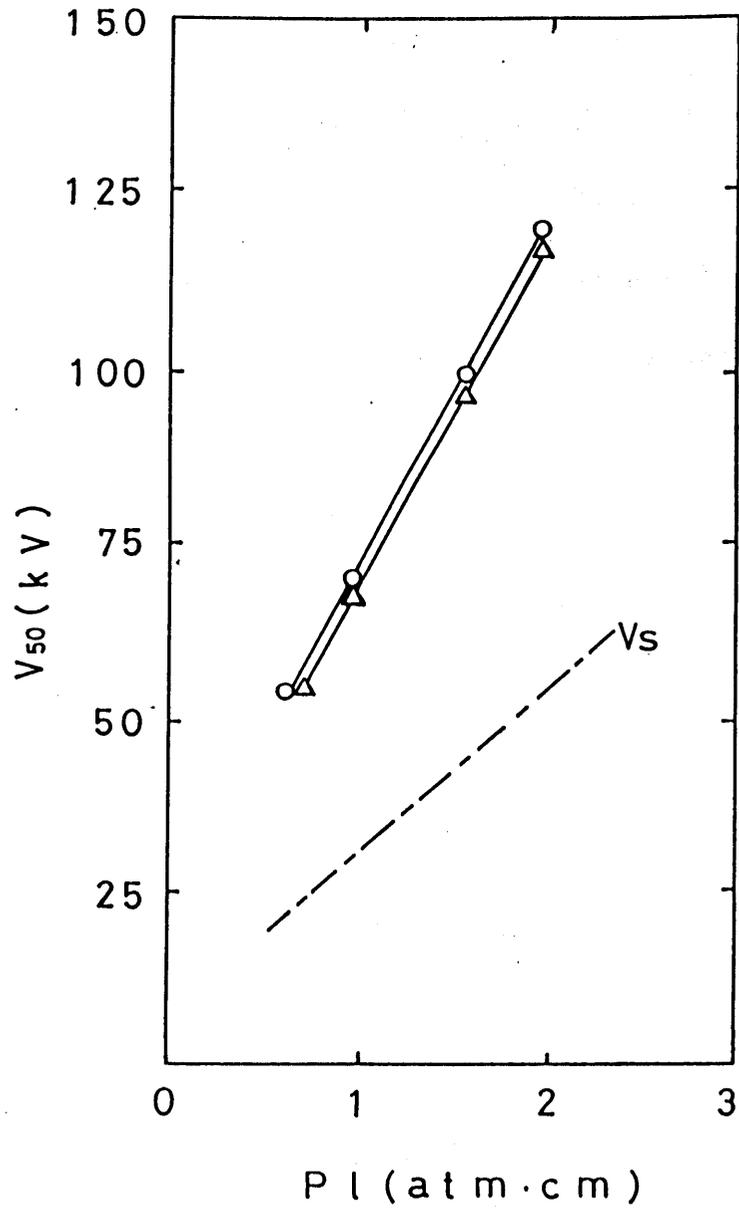
Fig. 6 50% probability of flashover voltage vs  $p l$  characteristics of  $N_2$
