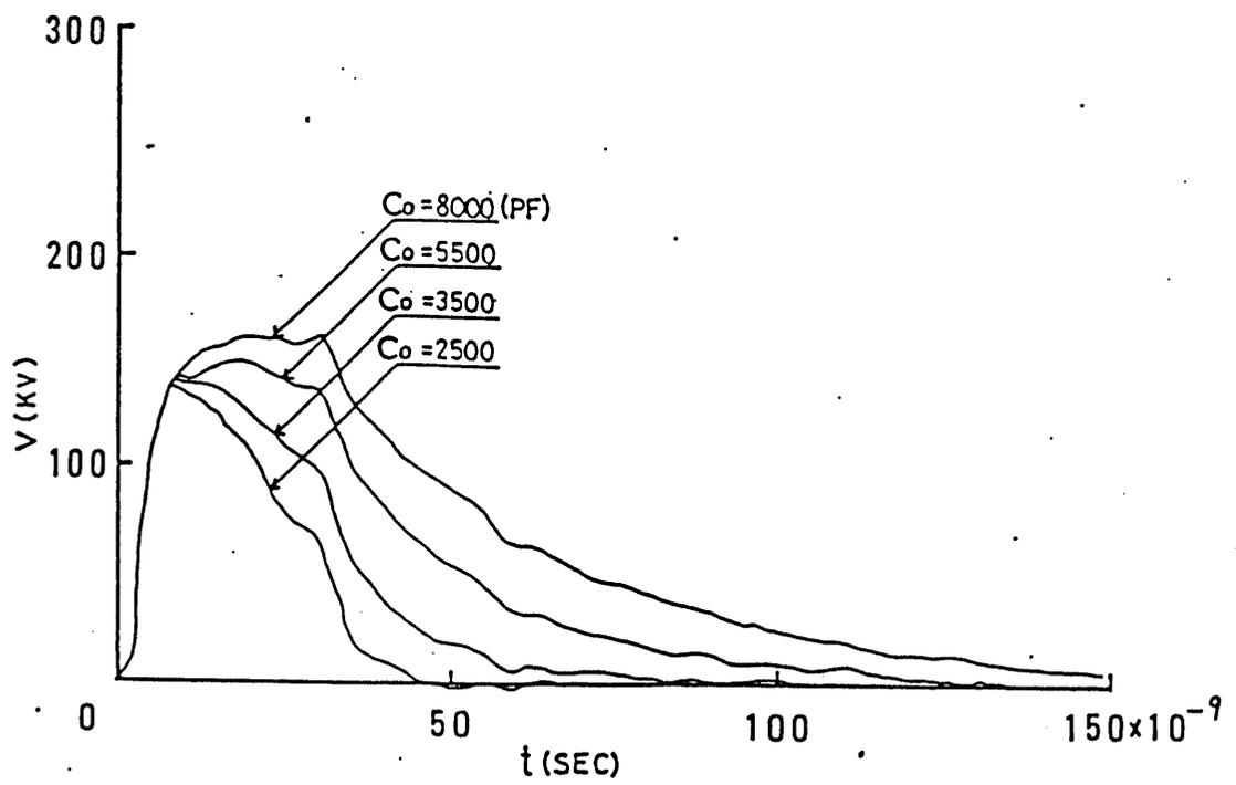
Fig. 6 Waveform analysis of CMG
