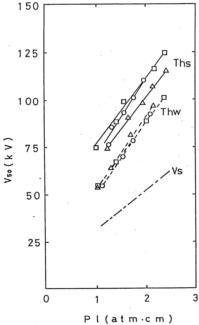
Fig. 7 50% flashover voltage vs  $p l$  characteristics
