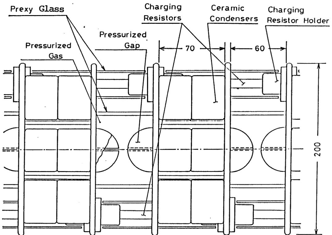
Fig. 2 Layout of the elements in unit module of CMG
