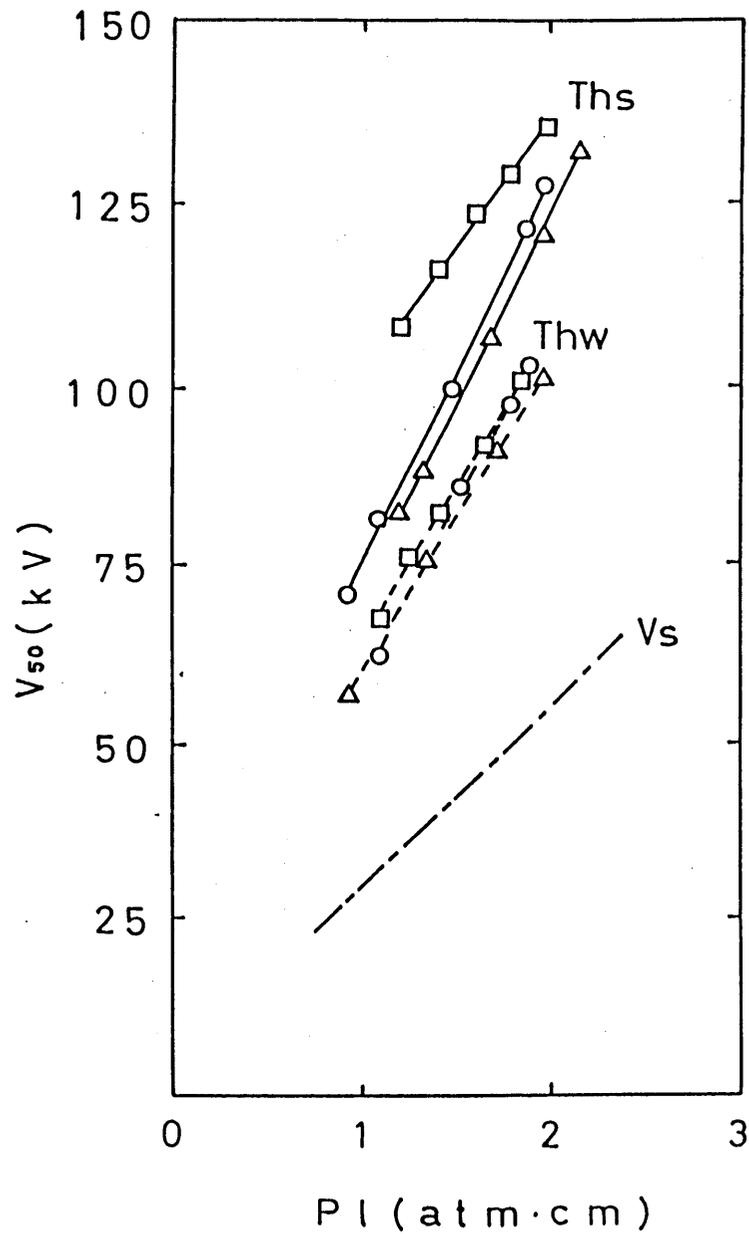
Fig. 3 50% flashover voltage vs  $p l$  characteristics of air
