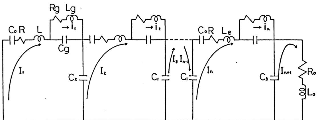
Fig. 5 The equivalent circuit of CMG with 6 stages
