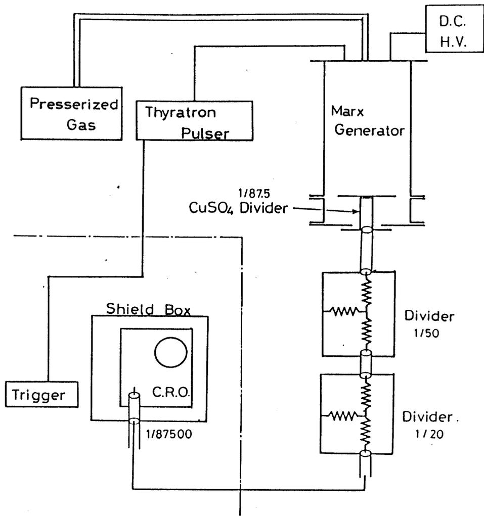
Fig. 3 The voltage measurement circuit
