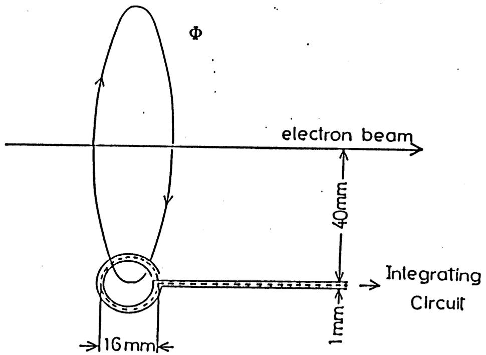
Fig. 9 Configuration arrangement of pick-up coil
