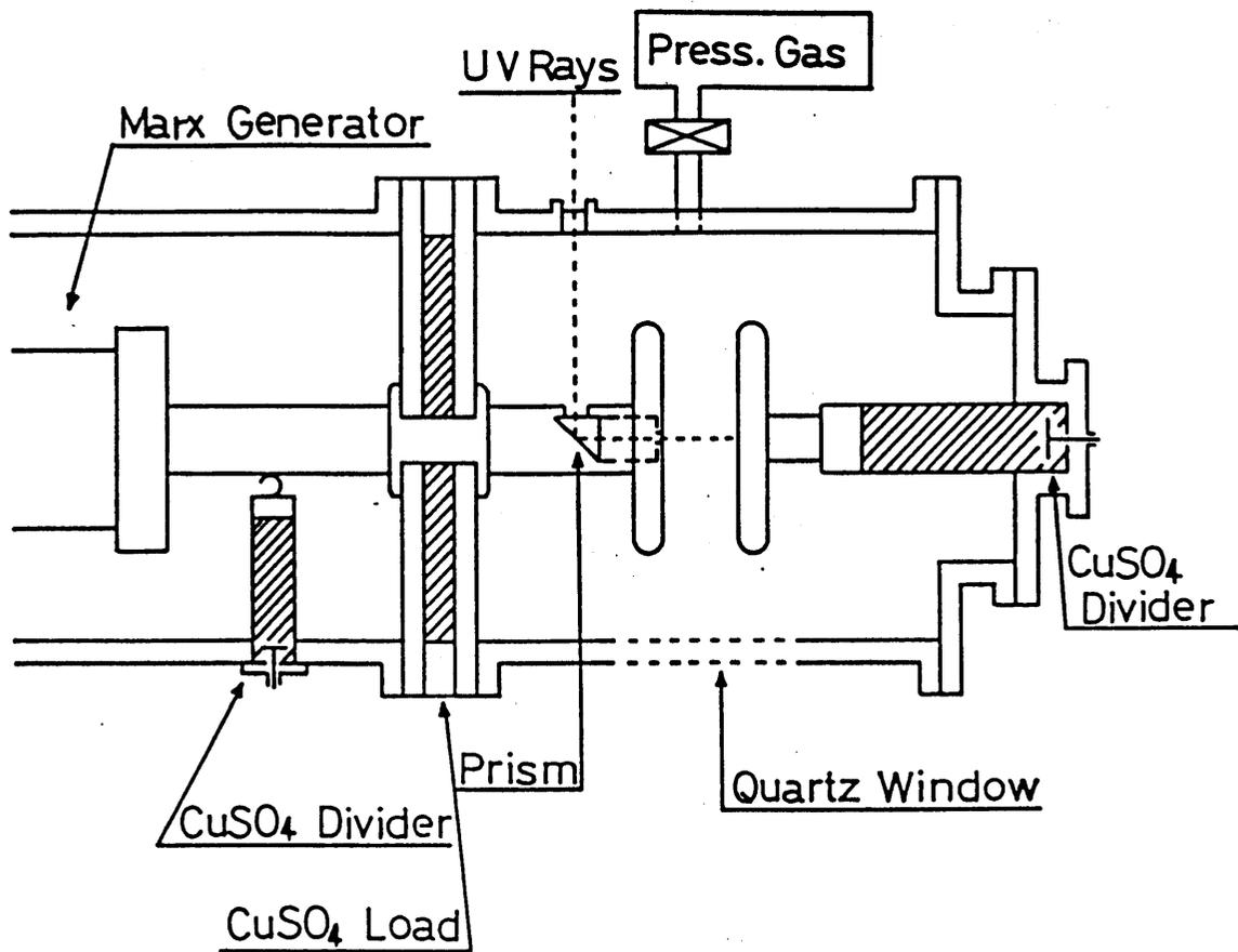
Fig. 2 Test gaps and illumination method of ultraviolet rays
