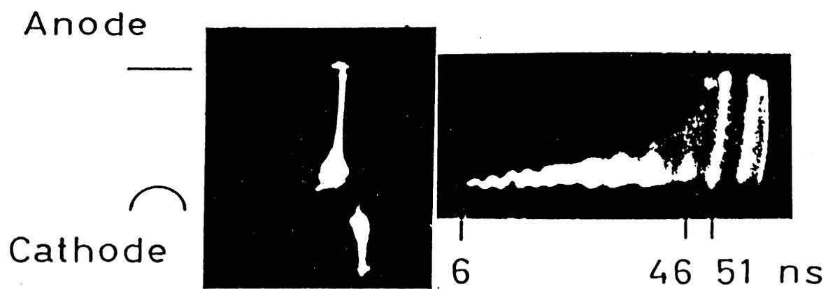
Fig. 5 Streak photograph in a nonuniform field
