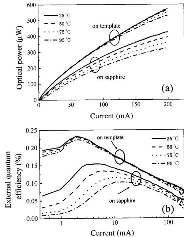
FIG. 5. Temperature dependence of light output power (a) and external quantum efficiency (b) versus current of LEDs on sapphire and on the template.
