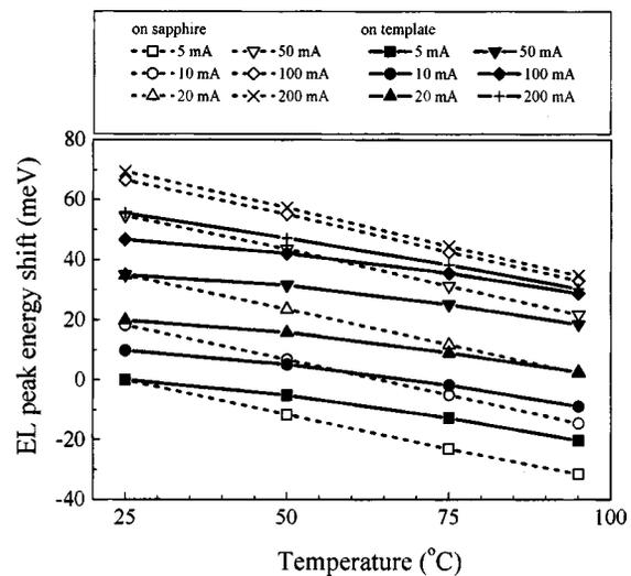
FIG. 7. EL peak energy shift versus ambient temperature at various driving currents. For a clear comparison, the relative shifts were calculated with respect to the peak energy at 5 mA and at an ambient temperature of 25 °C.
