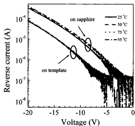
FIG. 4. Reverse  $\log(I)$ - $V$  characteristics of the LED dependent on ambient temperature (a) on sapphire substrate and (b) on AlN/sapphire template.
