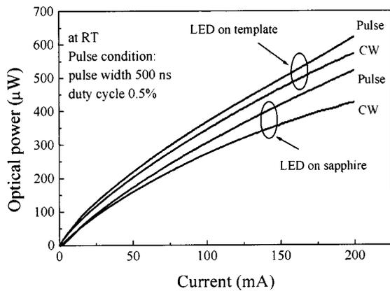
FIG. 6. A comparison of the typical  $L-I$  characteristics of the LEDs under pulsed and dc operation.
