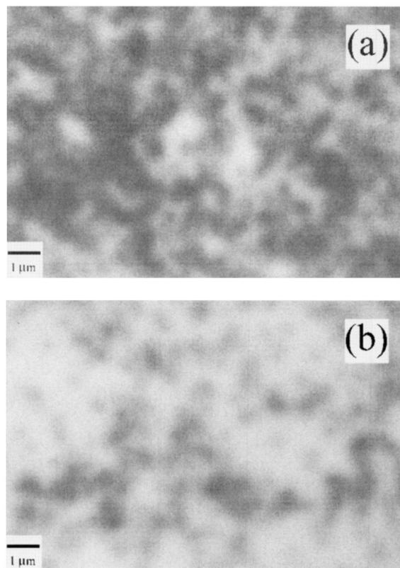
FIG. 2. EBIC images of InGaN MQW LED (a) on sapphire substrate and (b) on AlN/sapphire template.
