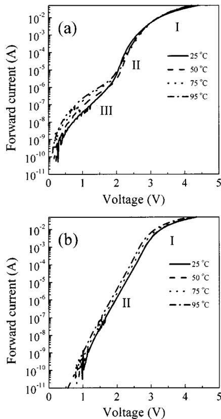
FIG. 3. Forward  $\log(I)$ - $V$  characteristics of the LED dependent on ambient temperature (a) on sapphire substrate and (b) on AlN/sapphire template.
