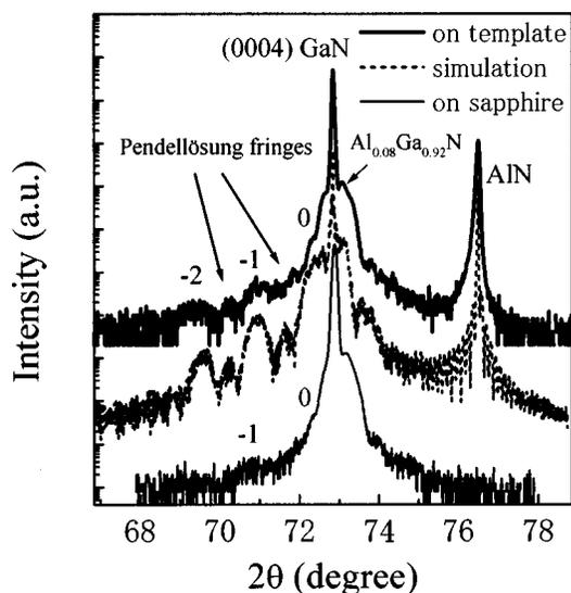
FIG. 1. A comparison of XRD rocking curves in GaN (0004)  $\omega$ - $2\theta$  scan mode between the LED on sapphire and on AlN/sapphire template.
