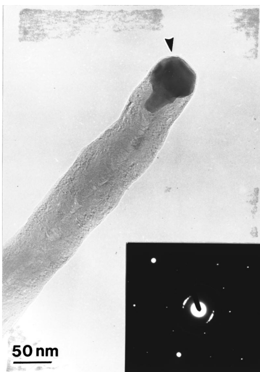
FIG. 4. TEM image of a Co-catalyzed CNT grown on a 30 \mu\text{m} wire by PECVD at 750 K; \text{C}_2\text{H}_2/\text{NH}_3=0.2/0.4 Torr. Inset: EDP from the CNT top region.
