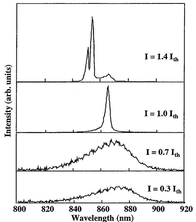
FIG. 9. Emission spectra of the  $\text{In}_{0.2}\text{Ga}_{0.8}\text{As}$  quantum dot-like laser on a Si substrate at different currents.
