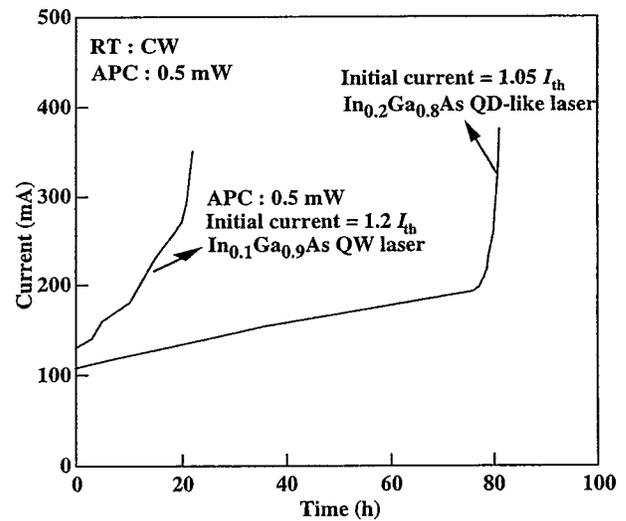
FIG. 12. Aging result of the  $\text{In}_{0.1}\text{Ga}_{0.9}\text{As}$  QW and  $\text{In}_{0.2}\text{Ga}_{0.8}\text{As}$  QD-like laser on a Si substrate at room temperature under the automatic power control condition.
