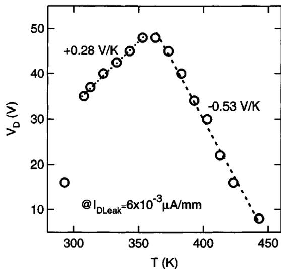
FIG. 4. Drain voltage ( $V_D$ ) of AlGaIn/GaN HEMTs at subthreshold regime ( $V_{GS} = -6.5$  V) for a fixed  $I_{DLeak}$  of  $6 \times 10^{-3} \mu\text{A}/\text{mm}$ .
