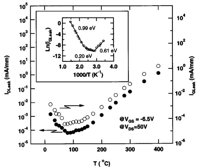
FIG. 3. Drain- and gate-leakage current of AlGaIn/GaN HEMTs for  $V_{DS} = 50$  V and  $V_{GS} = -6.5$  V (subthreshold regime). Inset figure activation energy plot of  $I_{GLEak}$  measured at  $V_{GS} = -6.5$  V.
