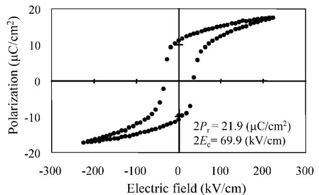
Fig. 3. Polarization hysteresis loops measured using SBT( $x=0.8$ ) dense ceramics at room temperature (25°C).
