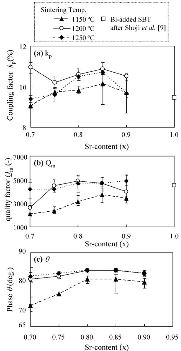
Fig. 6. (a) Electromechanical coupling factor in radial-extensional mode  $k_p$ , (b) mechanical quality factor  $Q_m$  and (c) phase  $\theta$  as a function of the composition ( $x$ ) for SBT ceramics sintered at  $1150$ – $1250^\circ\text{C}$ .
