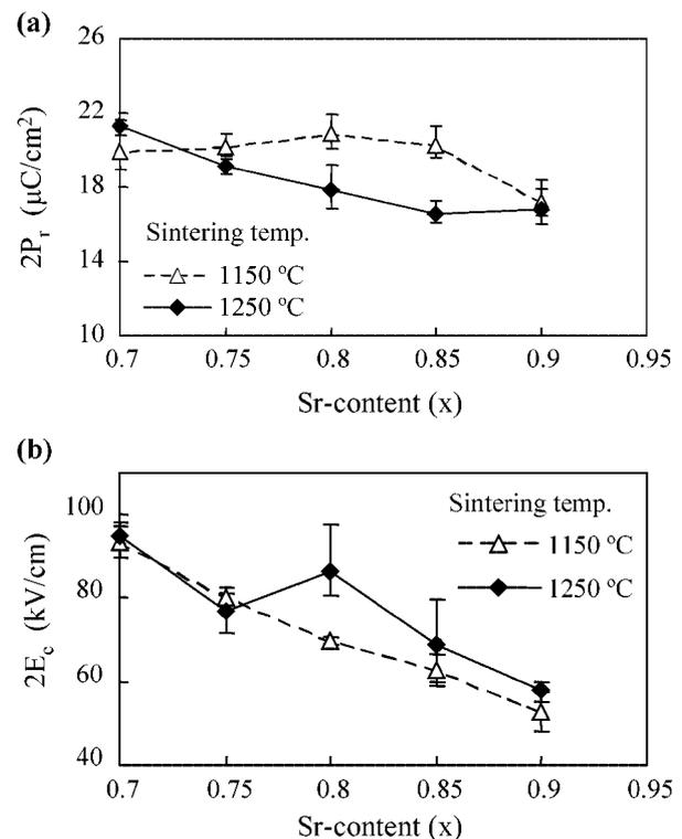
Fig. 4. (a) Remanent polarization  $2P_r$  and (b) coercive field  $2E_c$  as a function of the composition ( $x$ ) for SBT ceramics sintered at 1150 and 1250°C.
