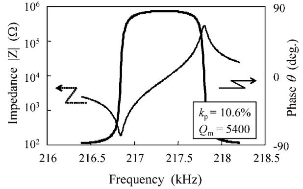
Fig. 5. Frequency dependence of impedance  $|Z|$  and phase  $\theta$  measured at room temperature in radial-extensional mode  $k_p$  for SBT ( $x=0.8$ ) ceramics sintered at  $1200^\circ\text{C}$ .
