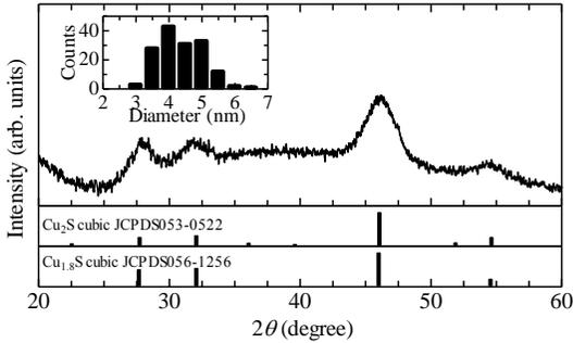
**Figure 1.** XRD pattern of  $\text{Cu}_{2-x}\text{S}$  NPs, with the standard diffraction data of cubic  $\text{Cu}_2\text{S}$  and  $\text{Cu}_{1.8}\text{S}$ . The inset shows the size distribution of NPs determined by STEM.
