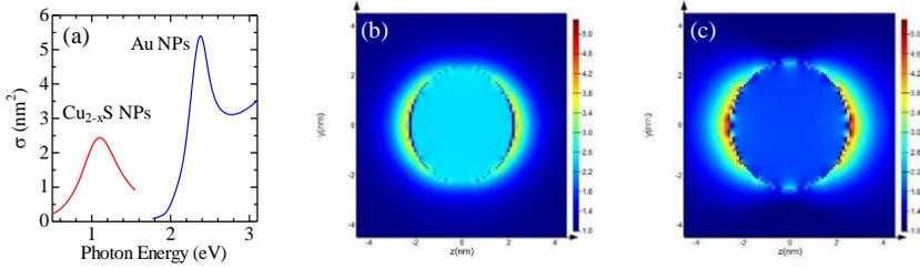
**Figure 4.** Results of the simulation by the FDTD calculations: (a) Absorption cross-section spectra near the LSPR calculated for a  $\text{Cu}_{2-x}\text{S}$  NP with a diameter of 4.5 nm in hexane (solid curve) and for an Au NP with a diameter of 5 nm in water (dotted curve). Electric field distribution around a single NP of (b)  $\text{Cu}_{2-x}\text{S}$  and of (c) Au upon irradiation by linearly polarized light with the respective resonance frequencies.
