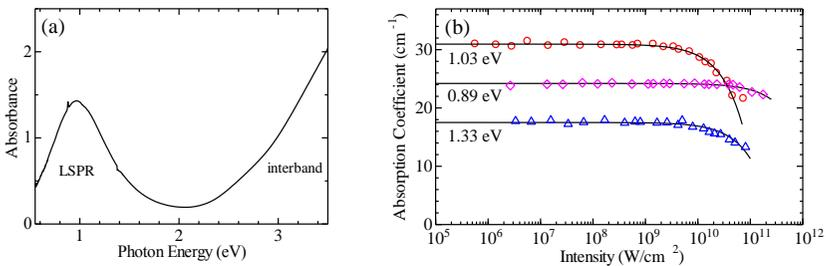
**Figure 2.** (a) Absorption spectrum of  $\text{Cu}_{2-x}\text{S}$  NPs dispersed in hexane. (b) Absorption saturation behavior of  $\text{Cu}_{2-x}\text{S}$  NPs, measured by incident laser pulses at various frequencies.
