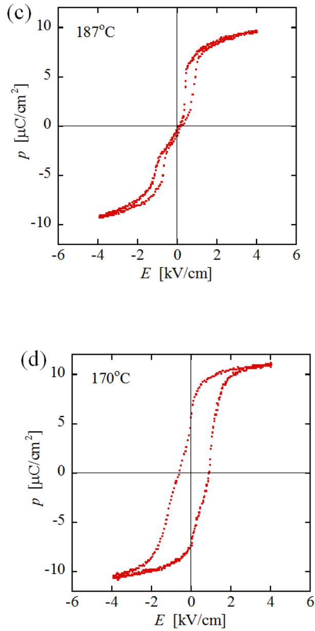
Fig. 2. P-E hysteresis loops under electric fields applied along  $[001]_c$  direction in PZN-9%PT, where frequency of the electric field is 6 Hz. Temperatures  $T$  are (a) 200, (b) 192, (c) 187, and (d) 170°C.
