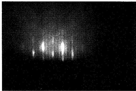
Fig. 2-3 Diffraction pattern from the GaSb (001)-(1×3) surface, the [110] azimuth, taken at an electron energy of 20 keV.
