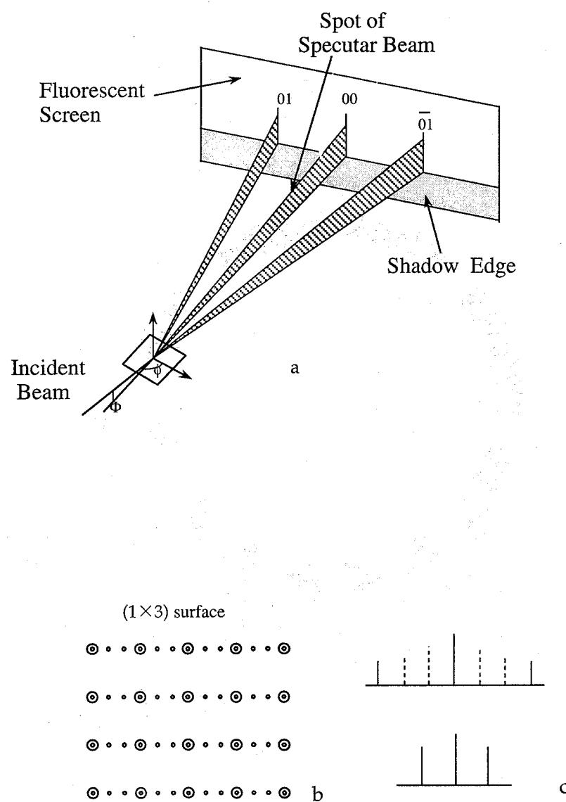
Fig. 2-2 Schematic diagram of RHEED geometry with grazing-angle incidence used as *in situ* analytical tool in MBE (a); Surface unit cell (b); diffraction patterns of  $(1 \times 3)$  reconstruction.
