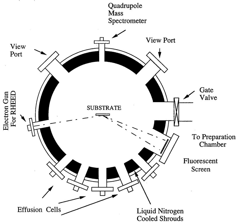
Fig. 2-1 Schematic cross-section of MBE growth chamber.
