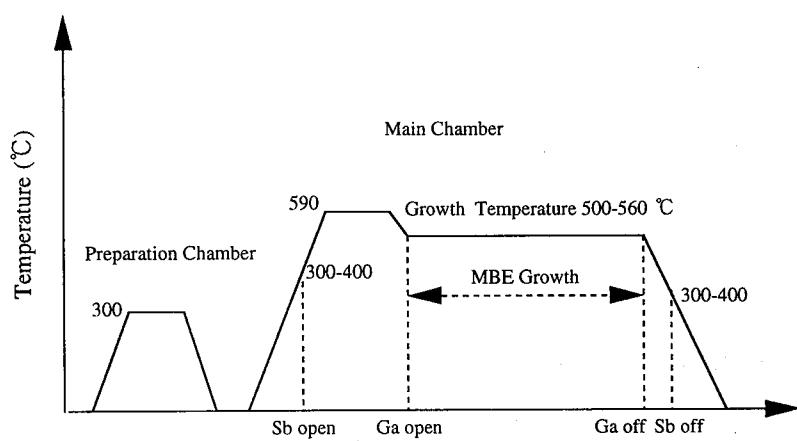
Fig. 2-4 Growth sequence of GaSb.
