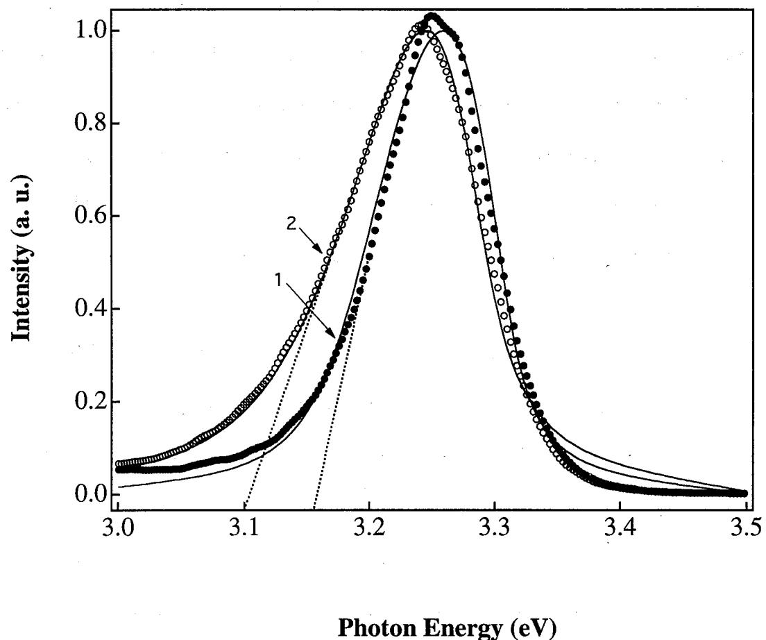
**Fig. 4-2** Normalized emission spectra of InGaN/AlGaN diode with two different injected current, (1) 1 A; (2) 3 A. The symbols are experimental data, and the solid curves represent theoretical results. The broken line in lower energy side is used to obtained  $E_g$  according to Tarucha's method.
