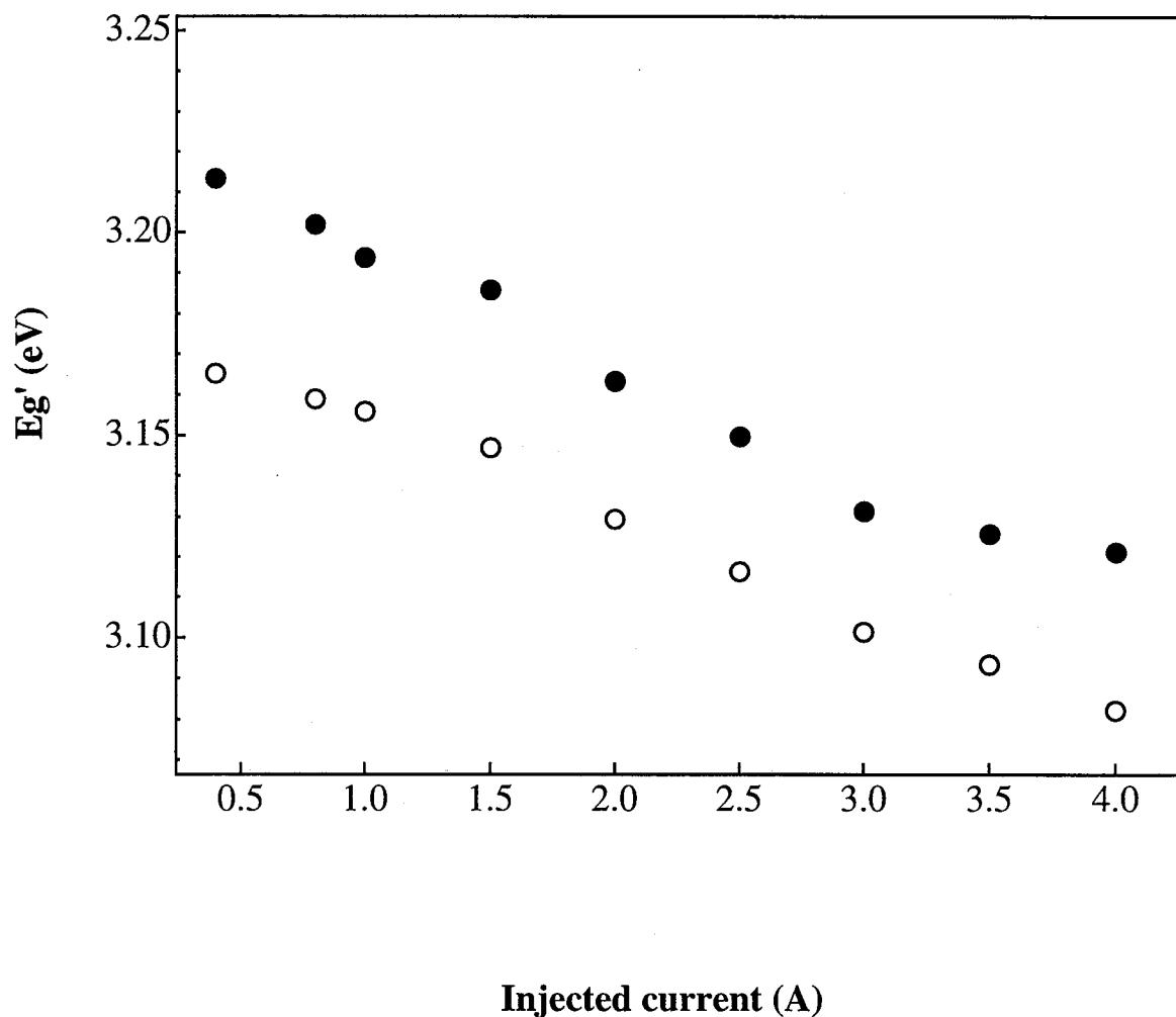
**Fig. 4-3** Injected current pulsed dependence of the renormalized  $E_g'$ . The dots are extracted from spectra line-shape fitting, and circles are obtained by Tarucha's method.
