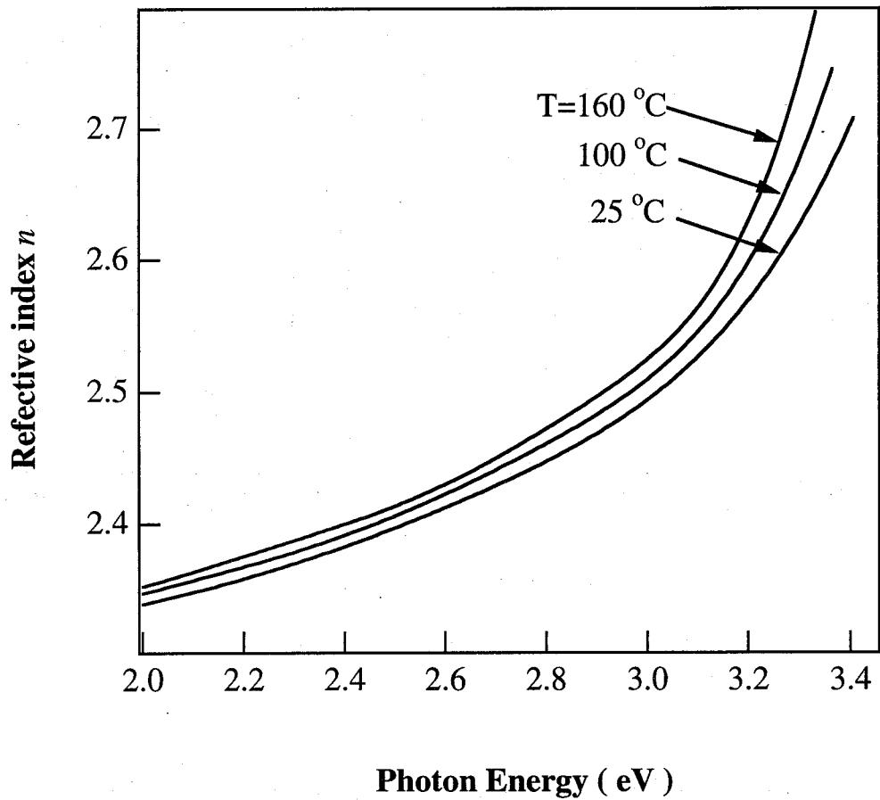
**Fig. 5-2 Refractive index of GaN for different temperatures.**
