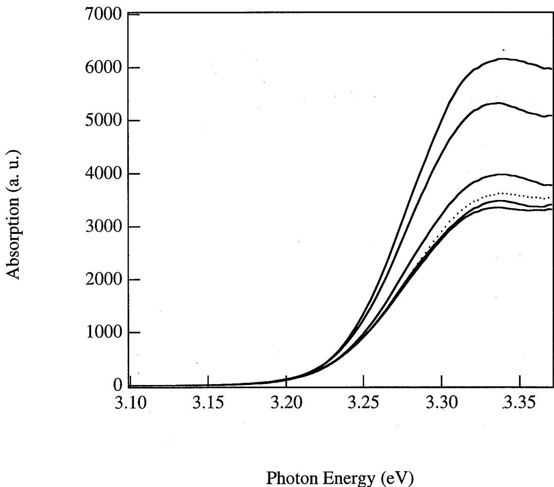
**Fig. 4-5** The calculated absorption spectra as functions of photon energy at different injected currents of (the current increasing from top to bottom) 1.5, 2.0, 2.5, 3.0, 3.5, and 4.0 A.
