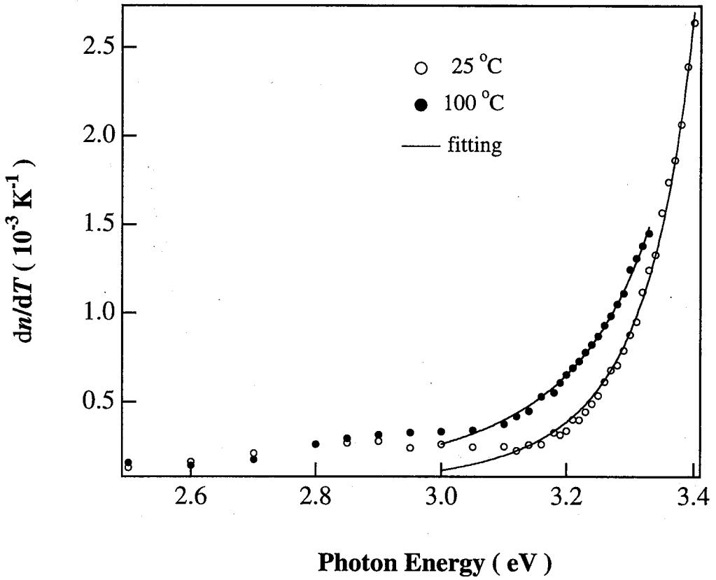
**Fig. 5-3 Thermo-optic coefficient of GaN in the band edge region for different temperatures**
