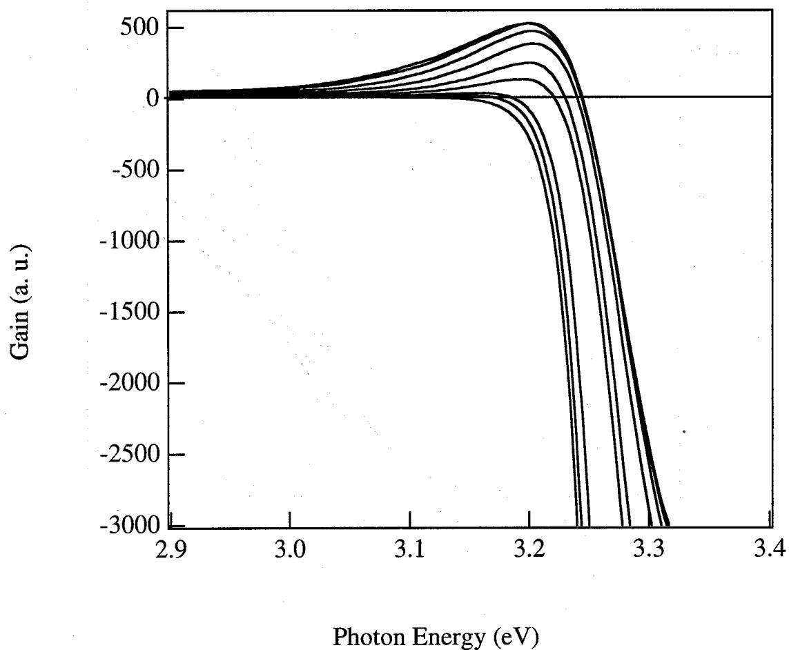
**Fig. 4-6** The calculated gain spectra as functions of photon energy at different injected currents of (the current increasing from bottom to top) 0.6, 0.8, 1.0 1.5, 2.0, 2.5, 3.0, 3.5, and 4.0 A.
