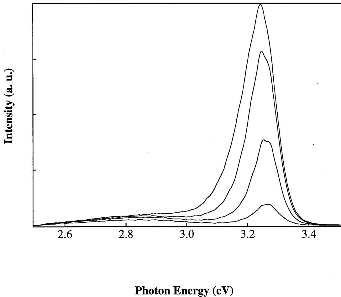
**Fig. 4-1** The experimental emission spectra as function of photon energy at different injected currents of (from bottom to top) 0.4, 1, 2, and 3 A.
