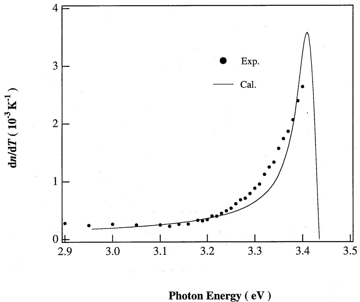
**Fig. 5-4** Photon energy dependence of thermo-optical coefficient of GaN. In the calculation of solid line, the experimentally obtained absorption coefficients (smoothed and interpolated for caculation) were used.
