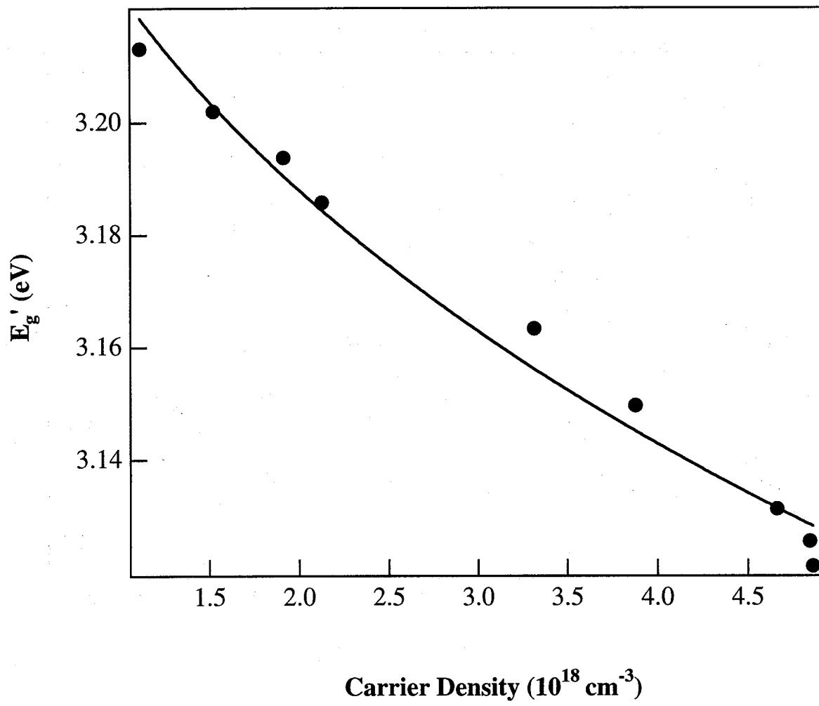
**Fig. 4-4** Renormalized  $E_g'$  as a function of carrier density. The dots represent spectra shape-line fit results, and the solid curve is for that calculated ones using  $E_g' = E_g - 5.8 \times 10^{-8} (n^{1/3} + p^{1/3})$  (eV) with  $E_g = 3.324$  eV.
