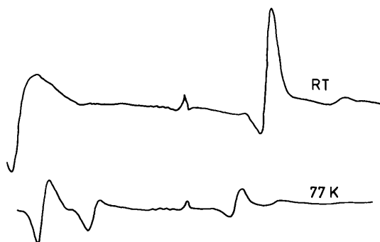
Fig. 4 X-band polycrystalline powder ESR spectra of [\text{Cu}(\text{CCl}_3\text{COO})_2(\text{caf})]_2 (2bz), (1), at room temperature(RT) and liquid nitrogen temperature(77K).
