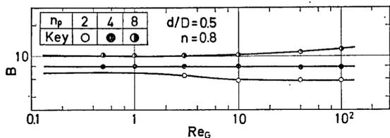
Fig. 4 Dependency of  $B$ -value on both modified Reynolds number and impeller blade number.
