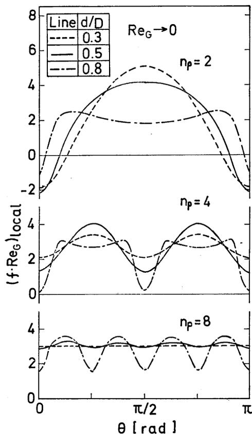
Fig. 3 Effect of impeller blade number on shear stress distribution at vessel wall.
