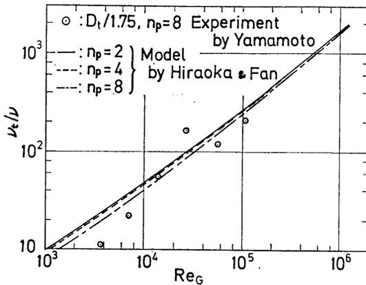
Fig. 6 Dependency of eddy kinematic viscosity on both modified Reynolds number and impeller blade number.
