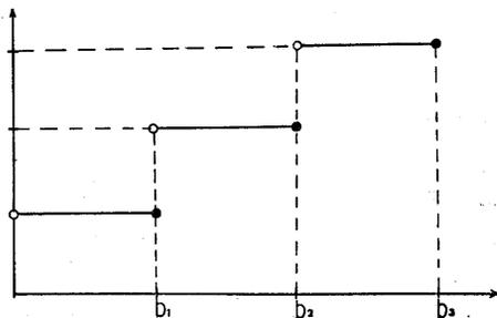
Fig. 1 Relationship between construction cost and traffic capacity  $b$
