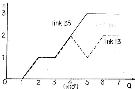
Fig. 5 Relationship between number of lanes n and traffic volume Q in the optimal network
