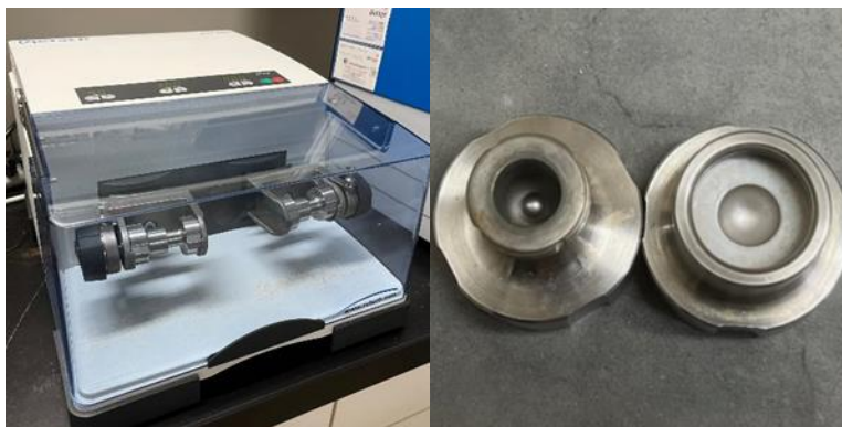
Figure S1. MM400, Retsch and stainless jar as well as ball used in this study.
