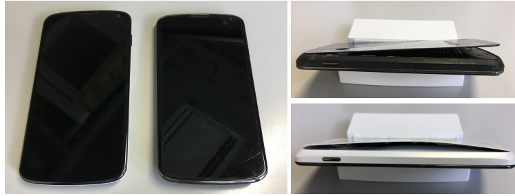
FIGURE 4.14: Two Nexus 4 devices used to run TaintDroid and IntelliDroid. Their batteries have been swollen in approximately one year of use.
