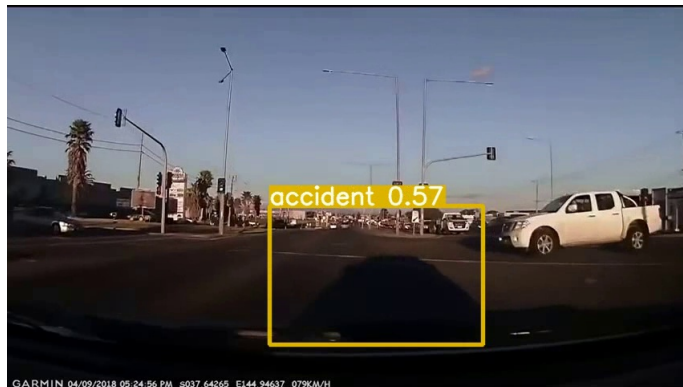
Figure 7.1: Example of the detection of the vehicle's shadow as the collided object.
