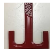
Fig.15 Photograph of new type impeller for viscoelastic fluid
