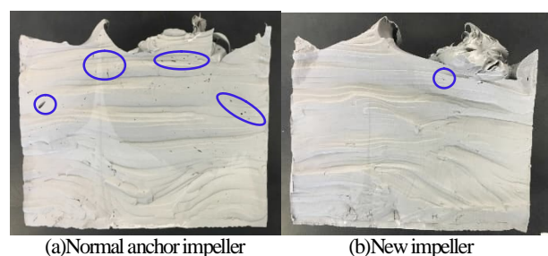
Fig.11 Mixing process of plastic fluid with new impeller in rotating vessel
