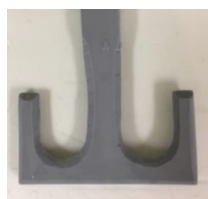
Fig.13 Photograph of prototype impeller for viscoelastic fluid
