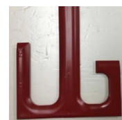
Fig.10 Photograph of new type impeller for plastic fluid
