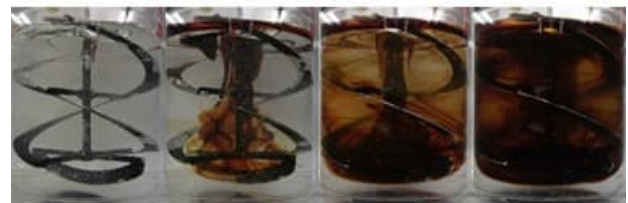
Fig. 14 Streak line of helical ribbon impeller with axis at Re = 0.60
