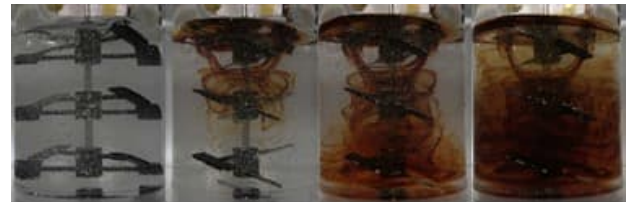
Fig. 12 Streak line of partial helical ribbon type at Re = 0.60
