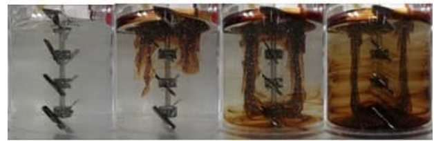
Fig. 13 Streak line of multiple pitched blade impellers type (4 stages) at Re = 0.60
