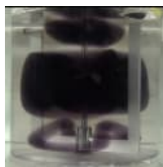
Fig. 1 Unmixed region of anchor impeller at Re = 6
