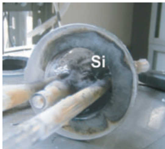
Fig. 4. An inner view of the top flange of reaction tube. The black part is mainly composed of crystalline silicon.
