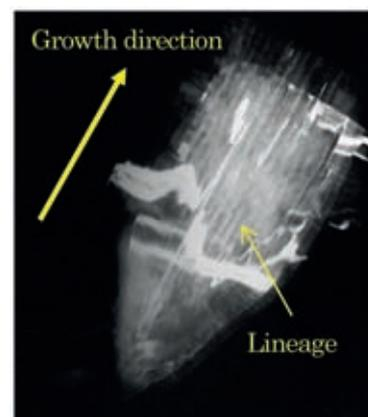
Fig. 15. X-ray topography of perpendicularly sliced Sapphire boule (diffraction : a(11-20))
