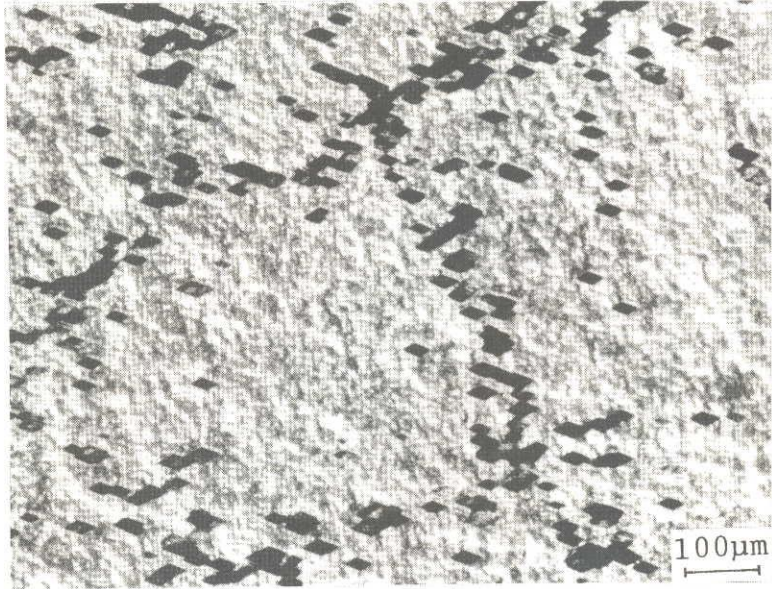
(a) LEC-grown GaAs substrate
