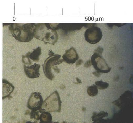
Fig. c-2 Microscopic photograph of the grinded unburnt PET particles
