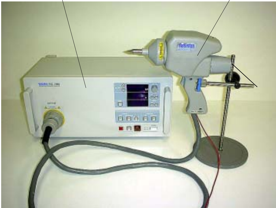
Figure 1.1: Appearance of a commercially available ESD-gun and its equipped high voltage generator.
