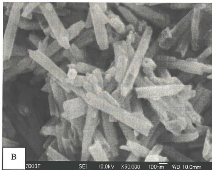
Figure 3.10 SEM images of ZnO nanotubes synthesized at 70 °C with the concentration of zinc ions 0.25 M
