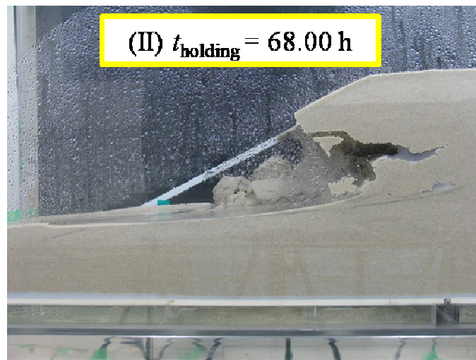
Fig. 3.1.14 Case (f), Progressive failure of the dike due to seepage and rainfall; t_{\text{holding}} = 68.00 h
