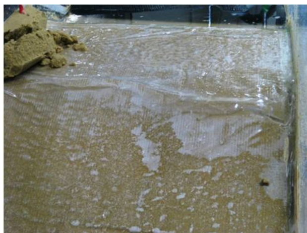
Fig. 3.1.2 Appearance of the downstream side slope after overflow; Case (1)
