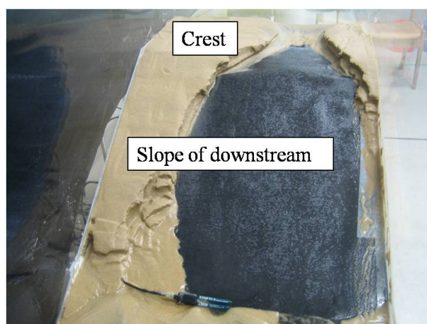
Fig. 3.1.12 Appearance of the downstream side slope after overflow; Case (2c)
