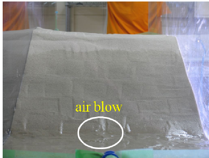
Fig. 3.1.11 Case (e), Slope of downstream; Holding test, Silica sand, without rainfall (just raising upstream water level)
