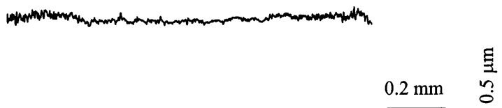
Fig. 4.12 Surface roughness of ball-shaped tool
