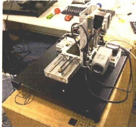
Figure 5.3: Originalmind 3-Axis Robot.
