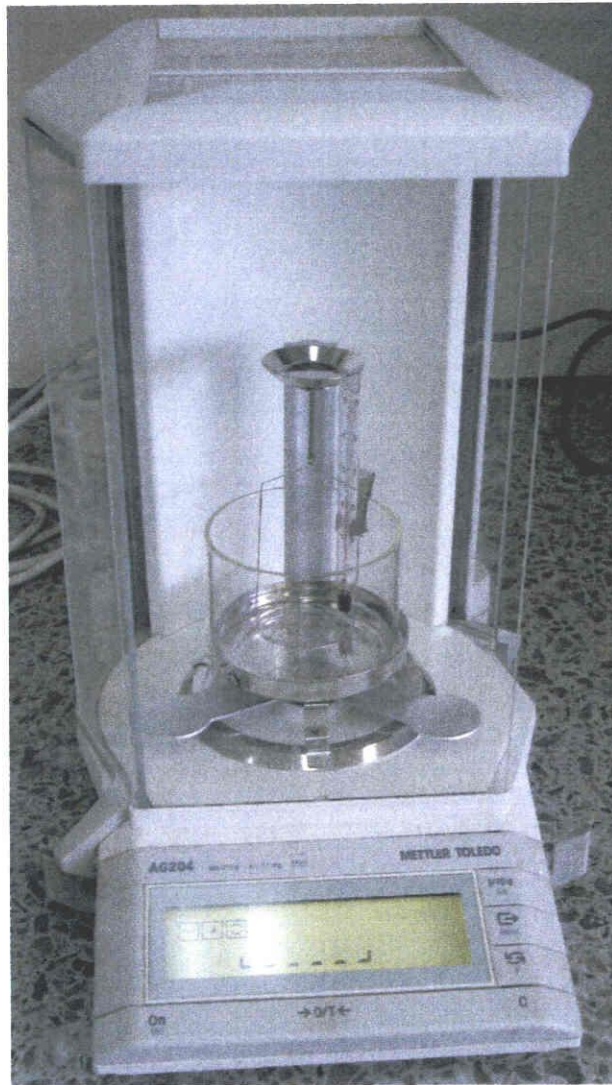
Figure 2.9 AG 206 Mettler Toledo density kit via archenemies principle
