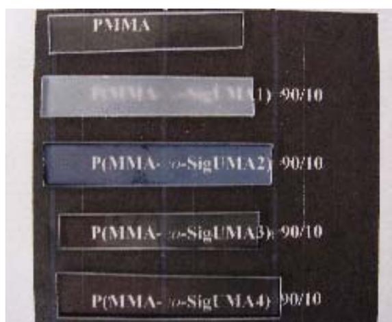
Fig. 2-3 Photographs of pure PMMA and P(MMA-*co*-SigUMAx) at 10 wt% of SigUMAx
