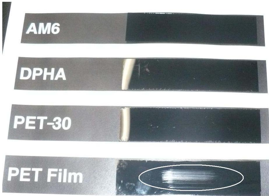
Fig.4-5 Film photographs of AM6 after scratch resistance test
