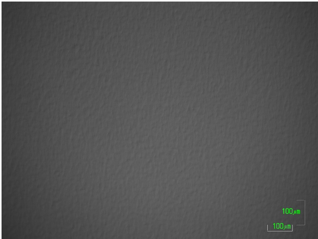
Fig. 6. 2. Optical Nomarski surface image of sample C with a 2 \mu\text{m} GaN epilayer.
