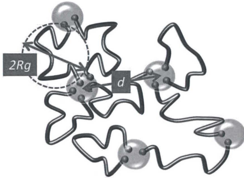
Figure 4.2. Illustration of a chain conformation in the PDMS gel
