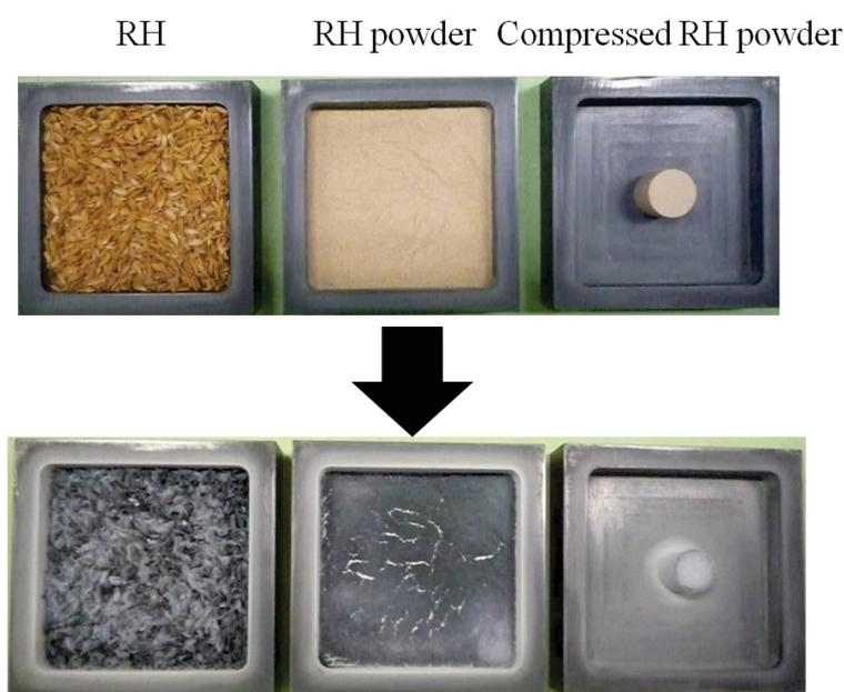
Fig. 2. 23 photo graphs of different raw RH materials and their pyrolyzed products.
