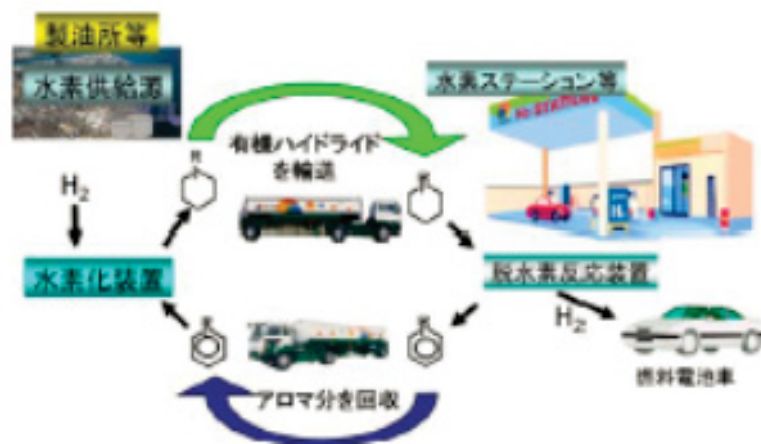
Fig. 1.5. Hydrogen storage system using organic hydride method.
