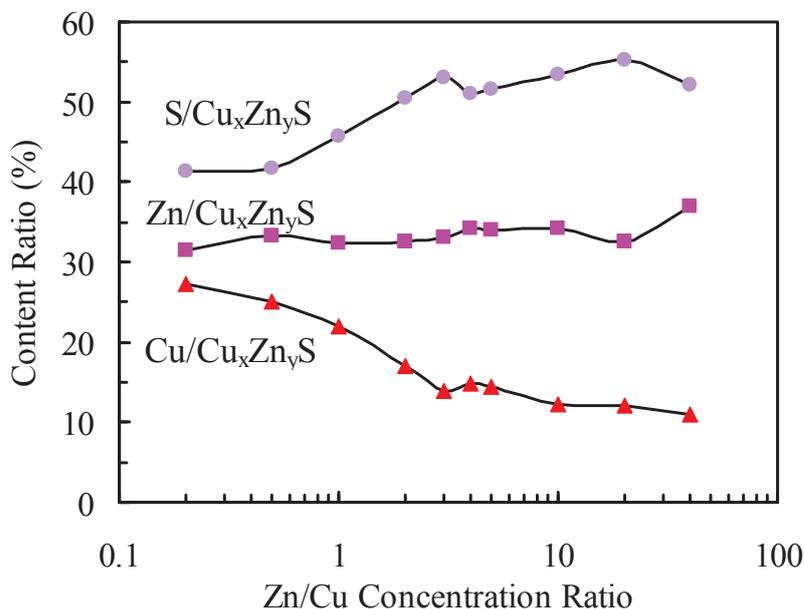
**Fig. 2.10. Relation between the Zn/Cu concentration ratio of the solution and the Cu, Zn, S content ratios of the deposited films.**
