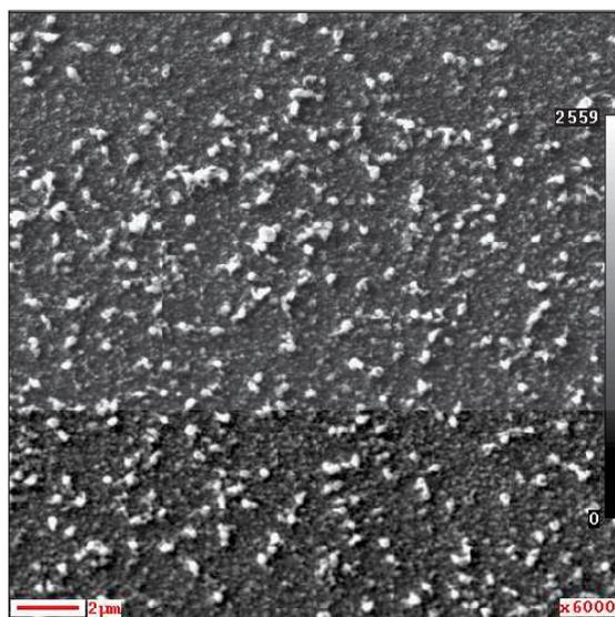
**Fig. 2.7. SEM photograph of the surface of the  $\text{Cu}_x\text{Zn}_y\text{S}$  film (Zn/Cu ratio in the solution = 4).**
