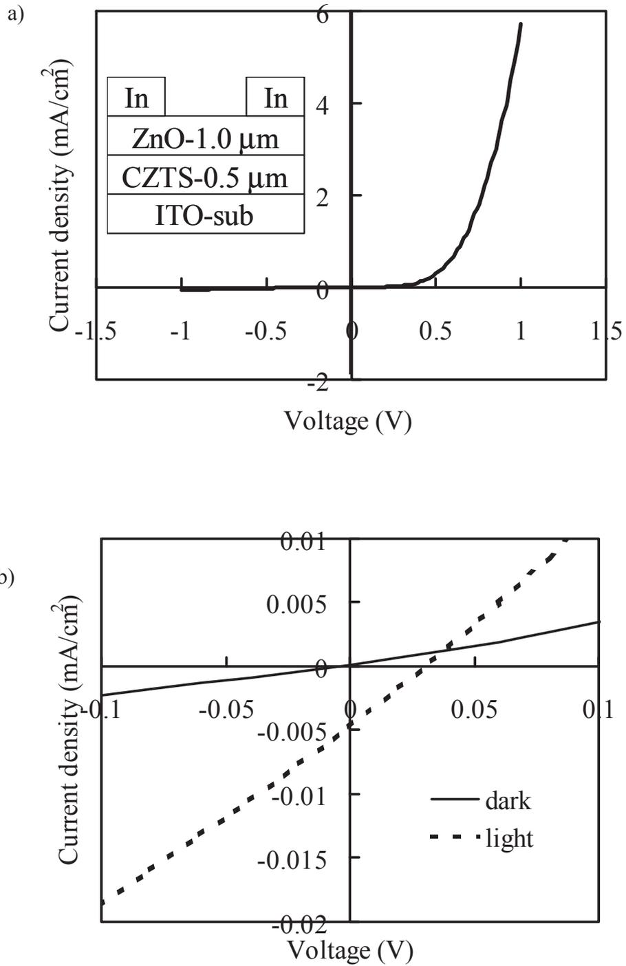
Fig. 3.20. a) I-V characteristics, and b) photovoltaic effect of the ZnO/sulfurized CZTS/ ITO heterojunction cells.
