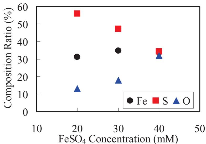
**Fig. 4.5. Composition of FeS<sub>x</sub>O<sub>y</sub> films deposited with different FeSO<sub>4</sub> concentrations.**
