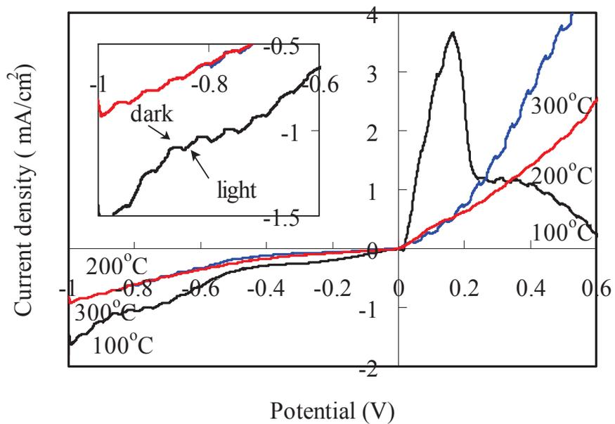
Fig. 4.17. PEC measurement results for the films annealed at 100, 200 and 300°C
