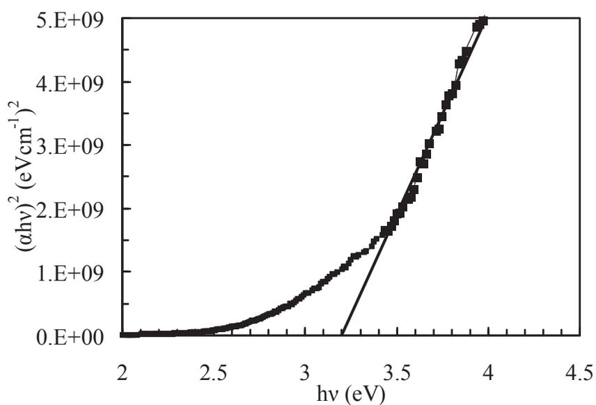
Fig. 2.14. Estimation of the band gap for the deposited  $\text{Cu}_x\text{Zn}_y\text{S}$  (Zn/Cu=4) thin film.
