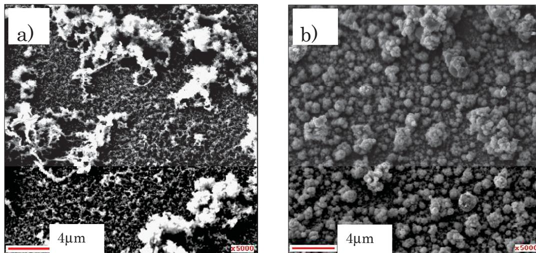
**Fig. 3.5.** SEM images of the surface of CZTSO (samples A and D)
