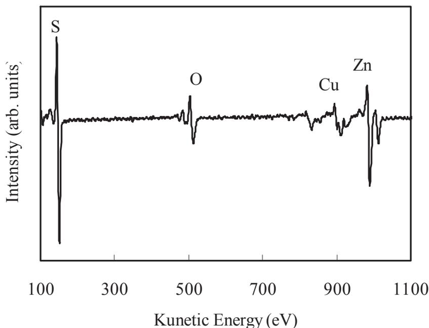
Fig. 2.17. AES spectra for the  $\text{Cu}_x\text{Zn}_y\text{S}$  thin film.
