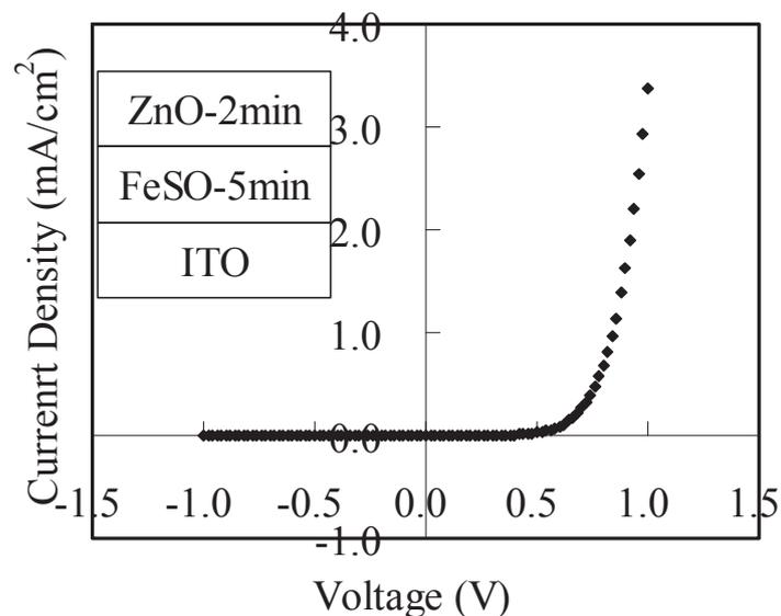
**Fig. 4.11. Current-voltage characteristics of the ZnO/  $\text{FeS}_x\text{O}_y$  / ITO heterojunction cell.**
