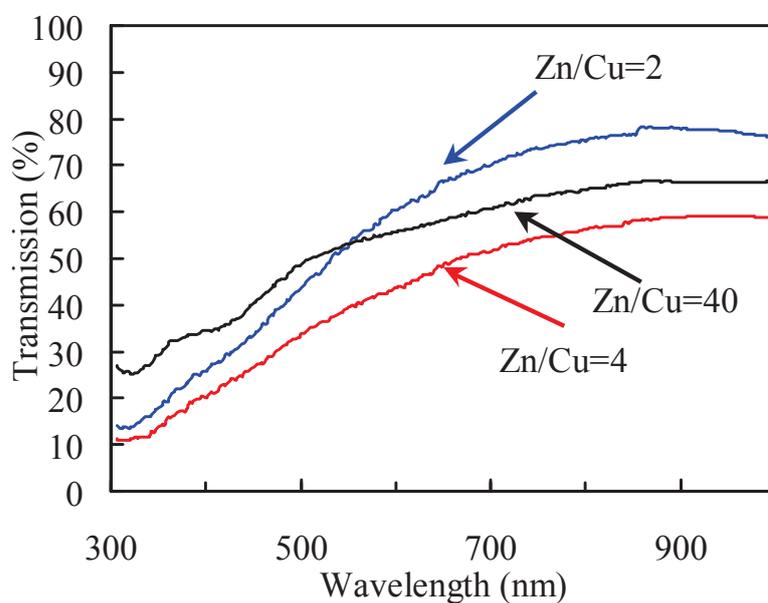
Fig. 2.13. Optical transmission spectra of the  $\text{Cu}_x\text{Zn}_y\text{S}$  thin films deposited with various concentration ratios (Zn/Cu=2, 4, 40).
