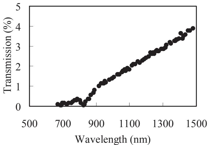
**Fig. 4.6. Optical transmission spectrum for the FeS<sub>x</sub>O<sub>y</sub> film.**
