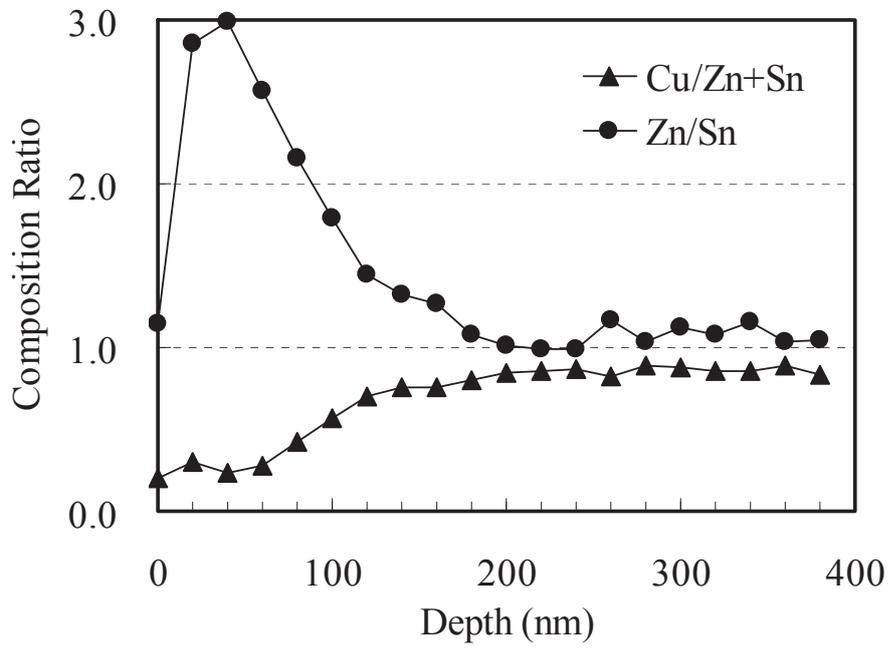
Fig. 3.13. AES spectra depth profiles for the sulfurized film.
