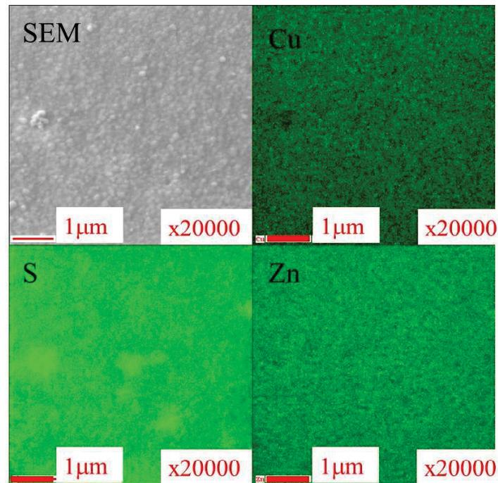
Fig. 2.18. SEM image and AES signal maps for Cu, Zn and S for the  $\text{Cu}_x\text{Zn}_y\text{S}$  film.
