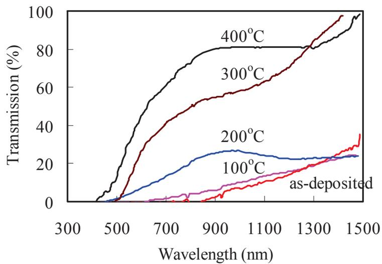
Fig. 4.14. Optical transmission spectra for the as-deposited films and the films annealed at different temperatures.
