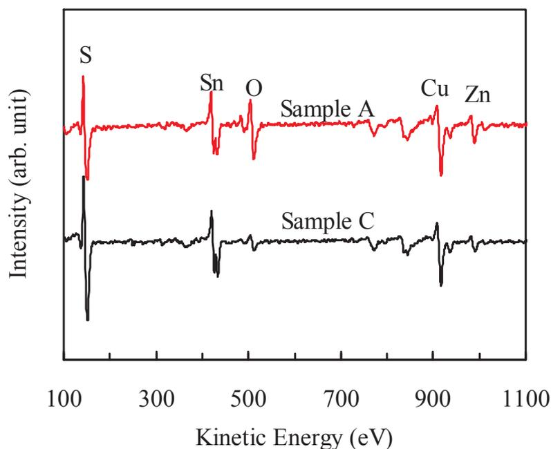
Fig. 3.3. AES spectra for samples A and C.
