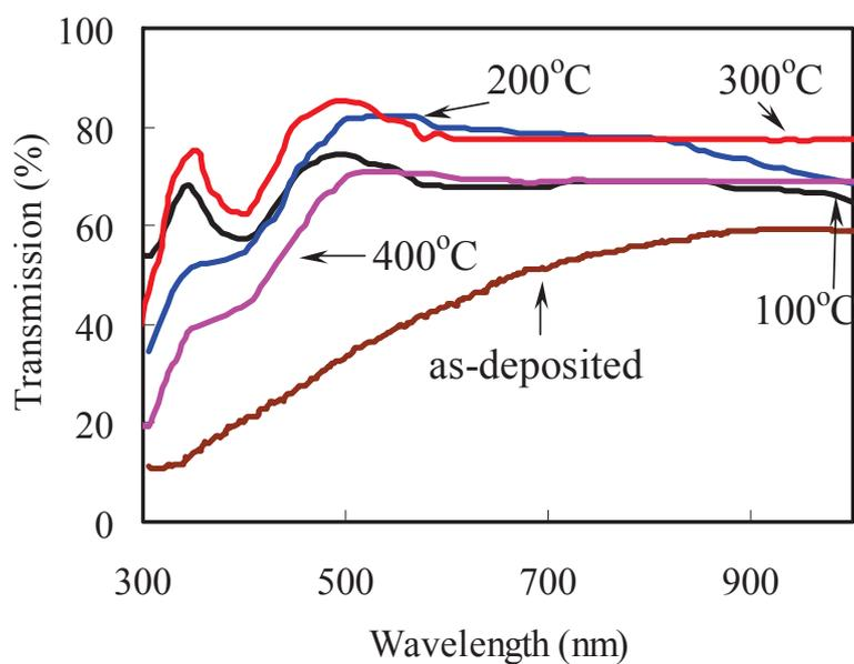
Fig. 2. 23. Optical transmission spectra for the as-deposited and annealed films.
