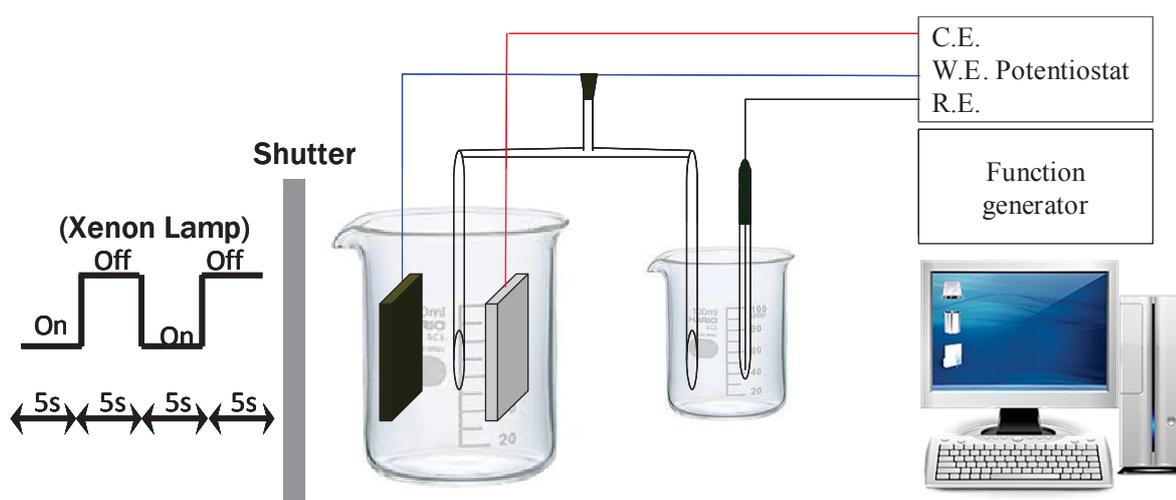
**Fig. 1.6. A schematic diagram of the 3-electrode cell apparatus used for photoelectrochemical (PEC) study of the deposited film.**
