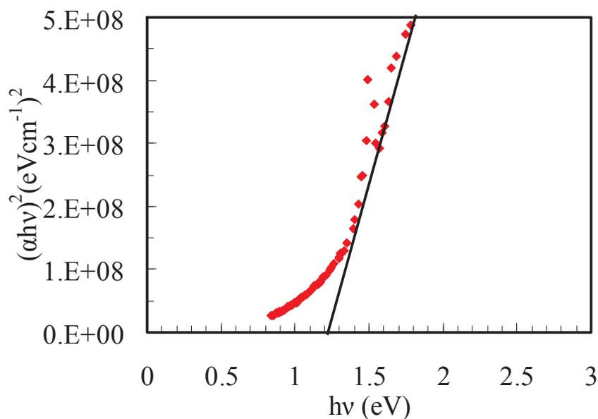
**Fig. 4.7. The bandgap estimation of the FeS<sub>x</sub>O<sub>y</sub> film.**
