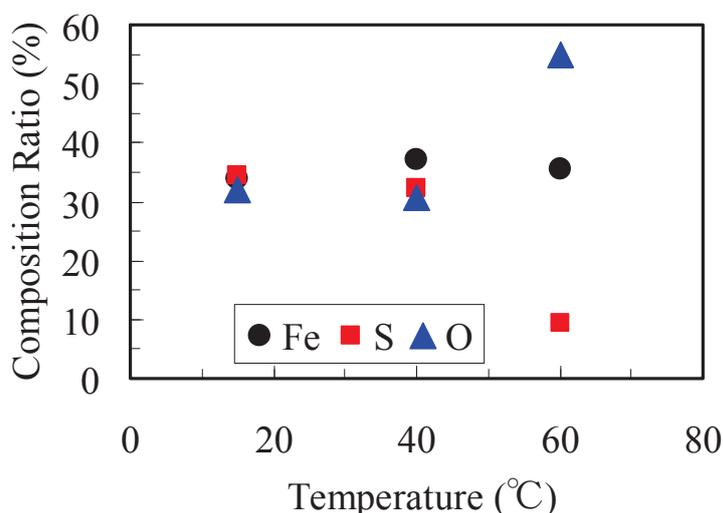
**Fig. 4.2. Composition of  $\text{FeS}_x\text{O}_y$  films deposited at different temperatures. (The potential was  $-0.8$  V, and the  $\text{FeSO}_4$  concentration 40mM).**
