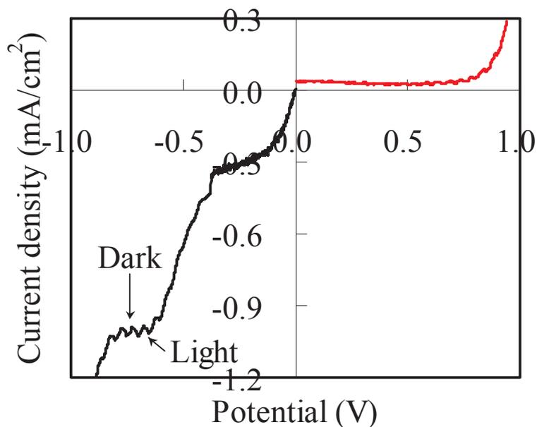
Fig. 4.8. PEC measurement results of the  $\text{FeS}_x\text{O}_y$  film.
