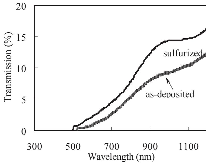
Fig. 3.16. Optical transmission spectra for the as-deposited and sulfurized films.
