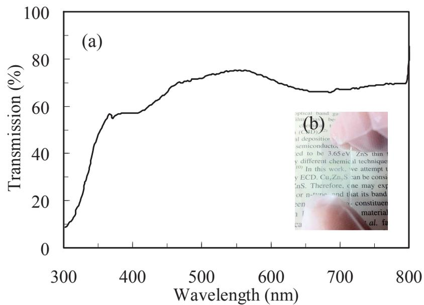
Fig. 2. 19. (a): Optical transmission spectra for the  $\text{Cu}_x\text{Zn}_y\text{S}$  film, (b): Photo of the  $\text{Cu}_x\text{Zn}_y\text{S}$  film.
