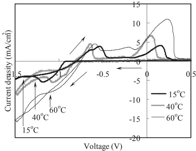
**Fig. 4.1. CV measurement for different solution temperatures 15°C, 40°C and 60°C (FeSO<sub>4</sub> concentration 40mM).**
