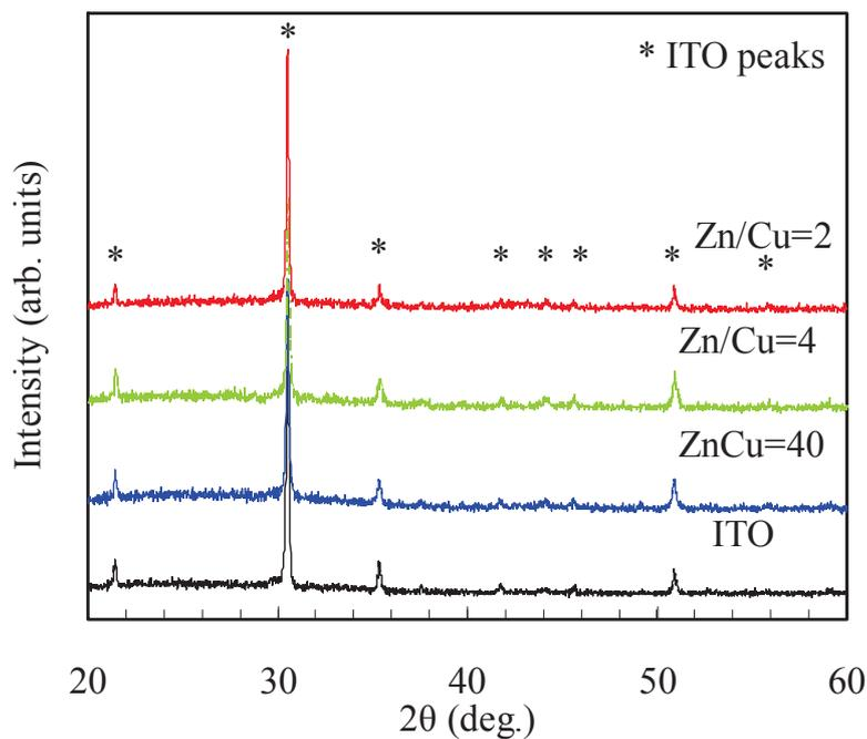
**Fig. 2.12.** XRD data of the  $\text{Cu}_x\text{Zn}_y\text{S}$  thin films of various concentration ratios ( $\text{Zn}/\text{Cu}=2, 4, 40$ ).
