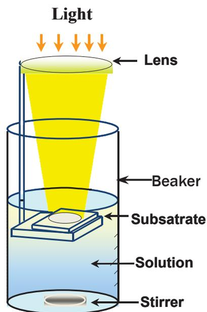
Fig. 1.2. Schematic diagram of the PCD method
