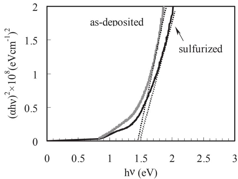
Fig. 3.17. Bandgap estimation of the as-deposited and sulfurized films.
