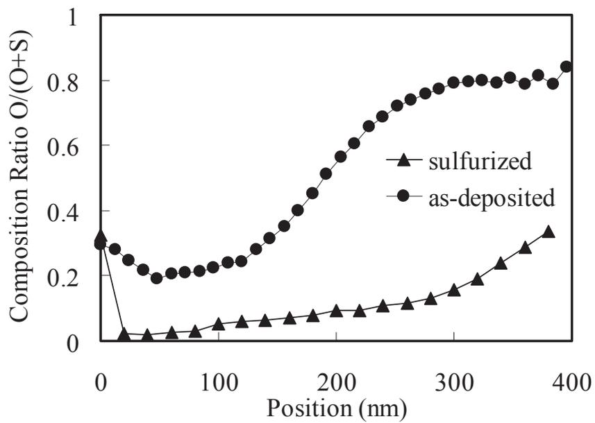
Fig. 3.14. Composition ratios O/(S+O) before and after sulfurization.
