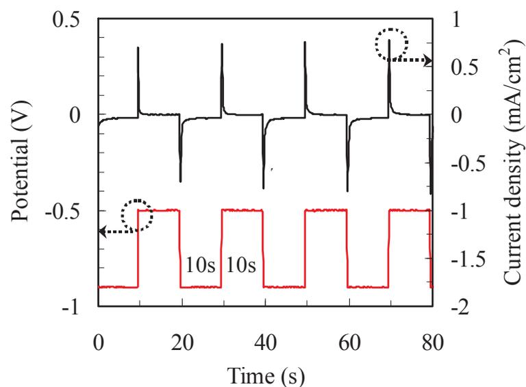
**Fig. 3.1.** Two-step pulsed voltage and current profile during deposition of sample C.
