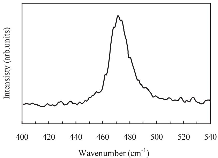
**Fig. 2.3.** Raman spectrum of the Cu<sub>x</sub>S thin film.
