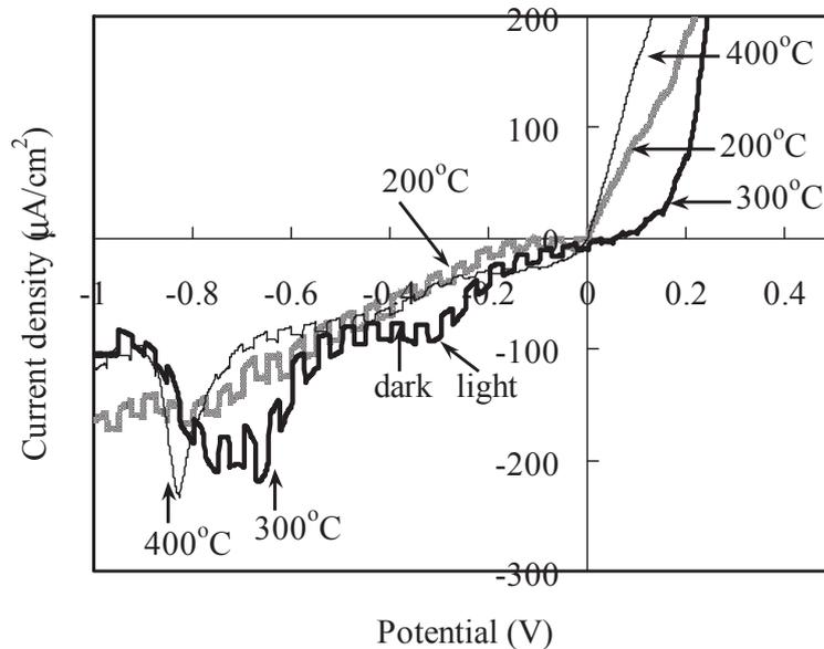
**Fig.2.25. PEC measurement results for the films annealed at 200 ~ 400°C**
