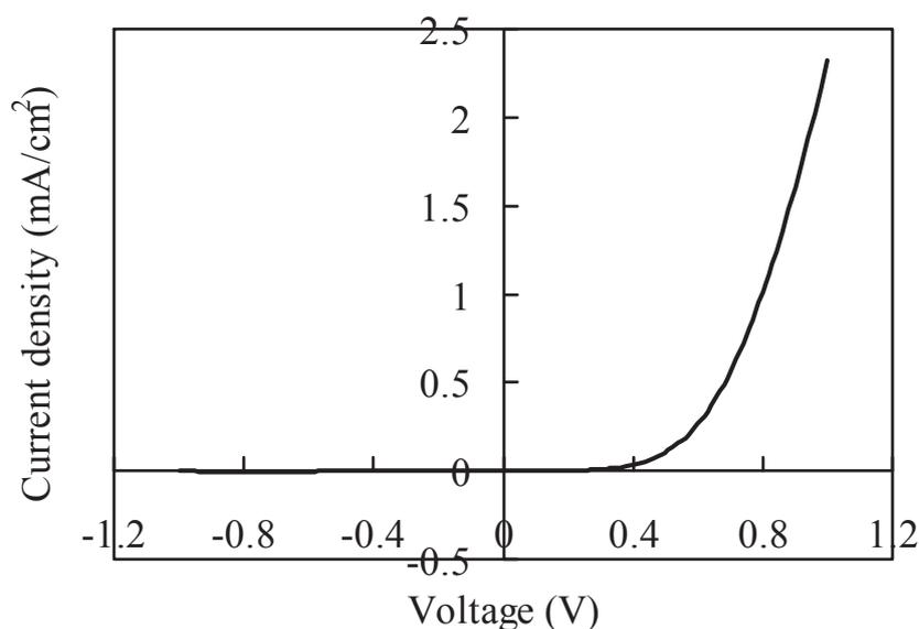
**Fig. 2.16. Current–voltage characteristics of the n-ZnO/p- $\text{Cu}_x\text{Zn}_y\text{S}$  (Zn/Cu=4) heterojunction.**
