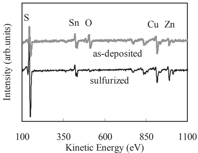
Fig. 3.11. AES spectra for the as-deposited and sulfurized films.
