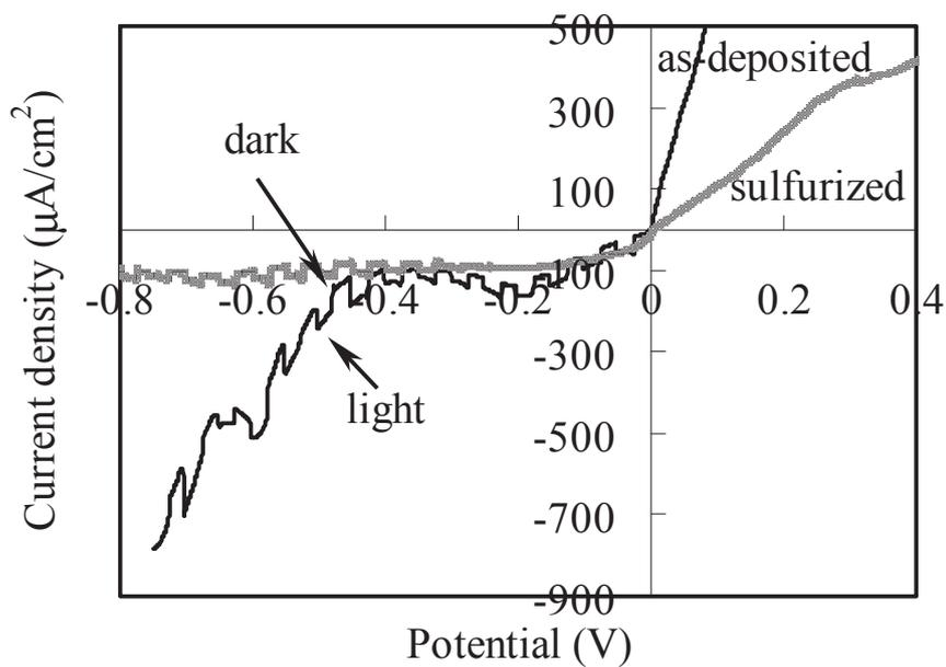
Fig. 3.19. PEC measurement results of the as-deposited and sulfurized films.
