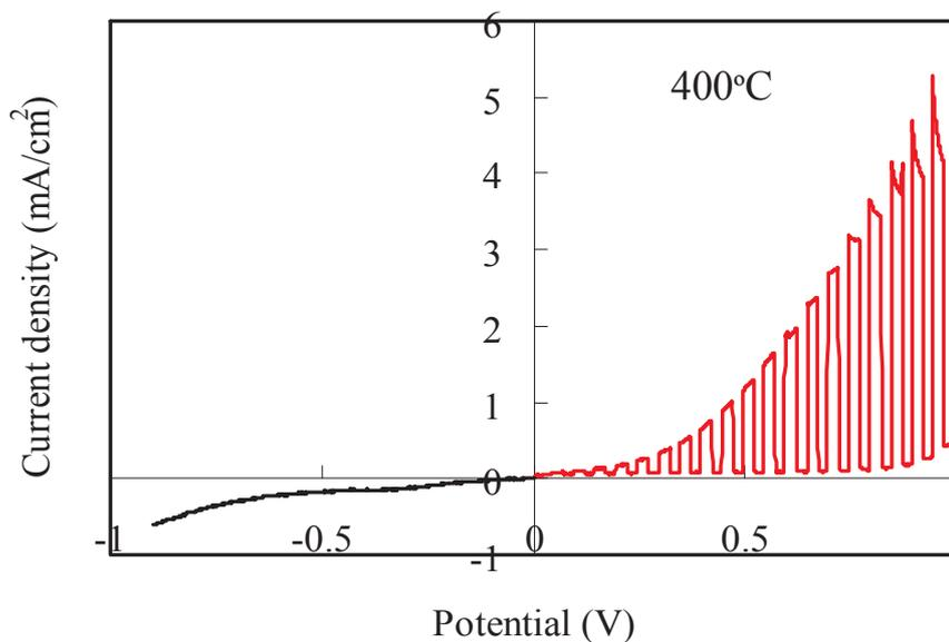
Fig. 4.18. PEC measurement result for the film annealed at 400°C.
