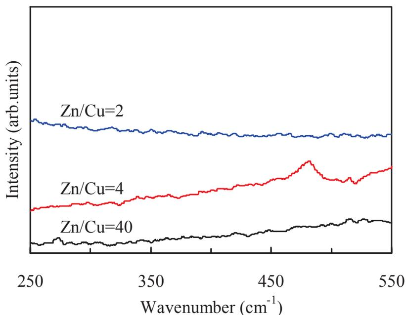
**Fig. 2.11. Raman spectra of the  $\text{Cu}_x\text{Zn}_y\text{S}$  thin films deposited with various concentration ratio ( $\text{Zn}/\text{Cu}=2, 4, 40$ ).**
