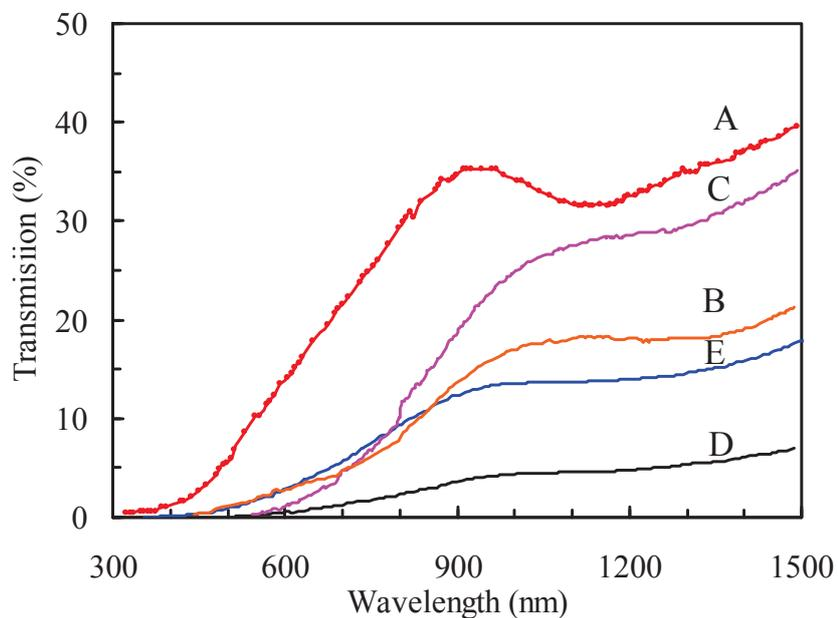
Fig. 3.6. Optical transmission spectra of the CZTSO samples (A, B, C, D, E).
