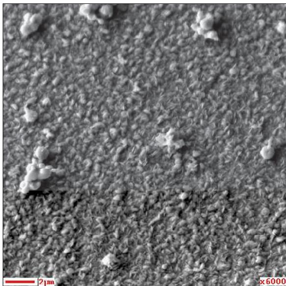
**Fig. 2.2.** SEM micrographs of the surface of the Cu<sub>x</sub>S thin film.
