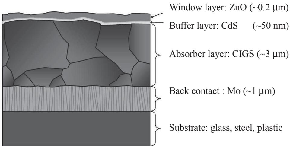
**Fig. 1.1. Schematic cross-sectional diagram of a thin film photovoltaic cell, showing the layers that comprise it.**
