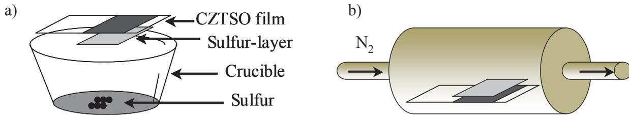
**Fig. 3.2. a) Schematic diagram of the sulfurization container, and b) Schematic diagram of the annealing furnace tube.**
