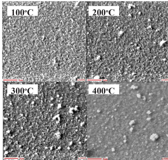
Fig. 4.13. The SEM image of the as-deposited film and the films annealed at different temperatures.
