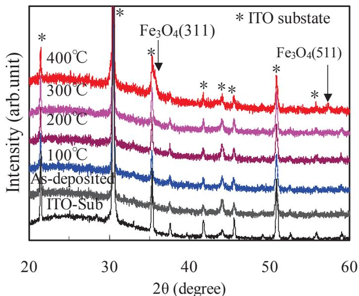
**Fig. 4.16. XRD spectra of the as-deposited films and the films annealed at different temperatures.**
