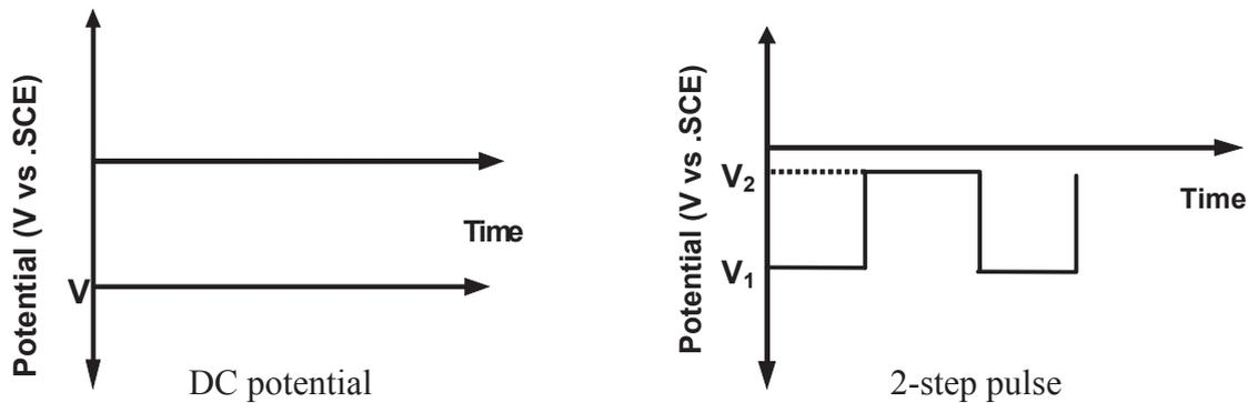
**Fig. 1.4. Electrochemical deposition techniques according to the nature of applied field.**
