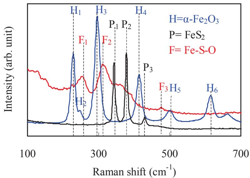
Fig. 4.10. Raman spectra of  $\text{FeS}_x\text{O}_y$ , hematite ( $\alpha\text{-Fe}_2\text{O}_3$ ), and pyrite ( $\text{FeS}_2$ ).
