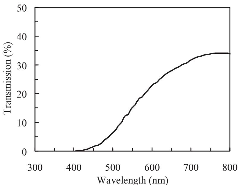
**Fig. 2.5. Optical transmission spectrum for the  $\text{Cu}_x\text{S}$  thin film.**
