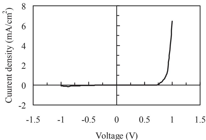
**Fig. 3.10** Current-voltage characteristics of the CZTSO/ ZnO/ ITO heterojunction cell (sample D).
