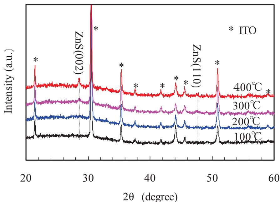
**Fig. 2. 24. XRD patterns of the  $\text{Cu}_x\text{Zn}_y\text{S}$  thin films at the various annealing temperatures.**
