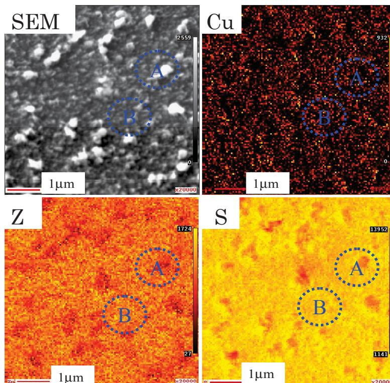
Fig. 2.8. SEM image and Auger signal maps for Cu, Sn, and S of the  $\text{Cu}_x\text{Zn}_y\text{S}$  film ( $\text{Zn}/\text{Cu} = 4$ ).
