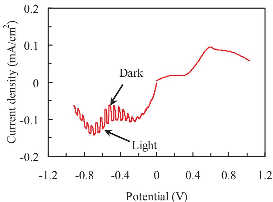
**Fig. 2.4. PEC measurement results for the  $\text{Cu}_x\text{S}$  thin film.**
