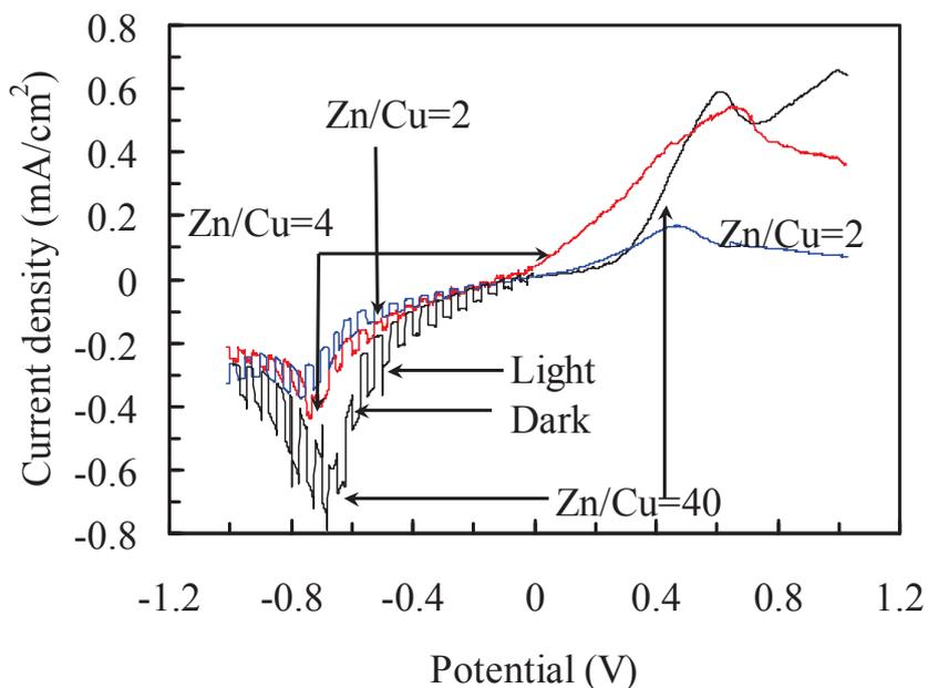
**Fig. 2.15. Results of the PEC measurement of the  $\text{Cu}_x\text{Zn}_y\text{S}$  thin films deposited with various concentration ratios (Zn/Cu=2, 4, 40).**
