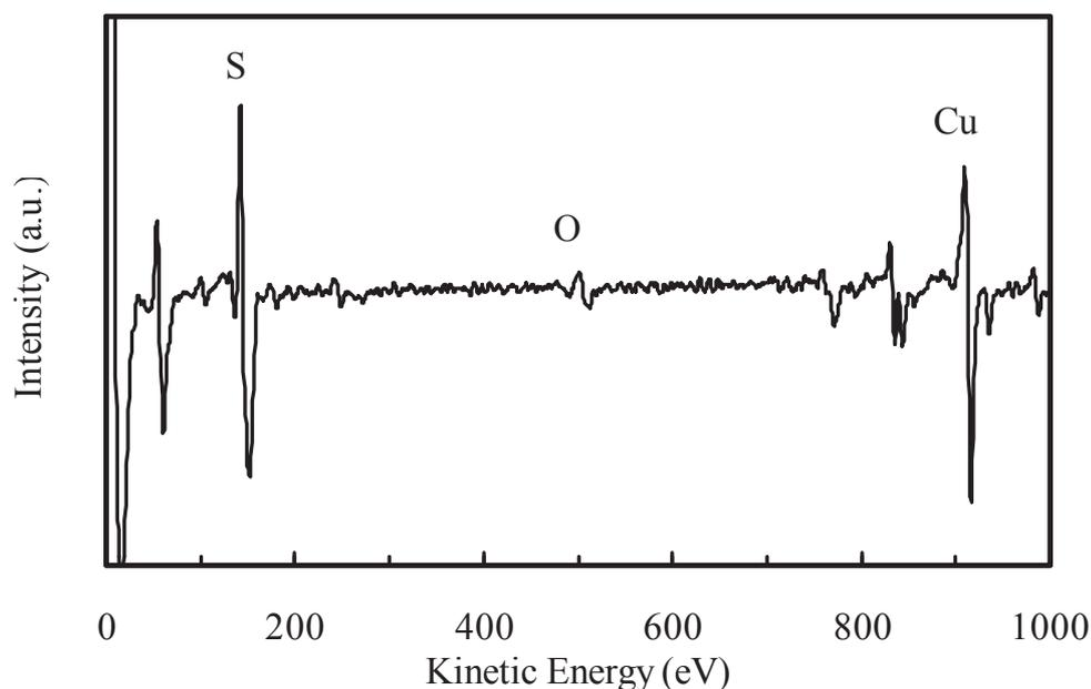
Fig. 2.1. AES spectra for the  $\text{Cu}_x\text{S}$  thin film.
