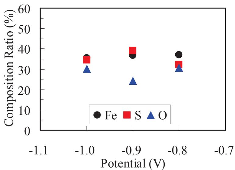
Fig. 4.4. Composition of FeS<sub>x</sub>O<sub>y</sub> films deposited at different potentials.
