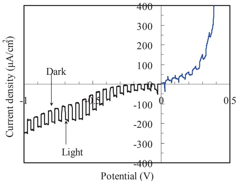
**Fig. 2. 20. PEC measurement results for the  $\text{Cu}_x\text{Zn}_y\text{S}$  film.**
