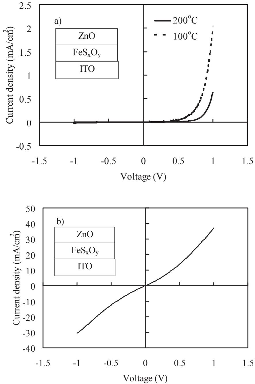
Fig. 4.19. I-V measurement of the ZnO/ annealed FeS<sub>x</sub>O<sub>y</sub> / ITO heterojunction cells with the FeS<sub>x</sub>O<sub>y</sub> films annealed a) at 100°C and 200°C, and b) at 300°C.
