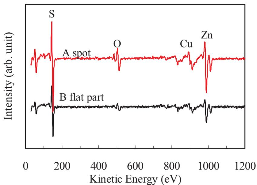
Fig. 2.9. AES spectra at position A (particle) and B (flat part) of the AES maps.
