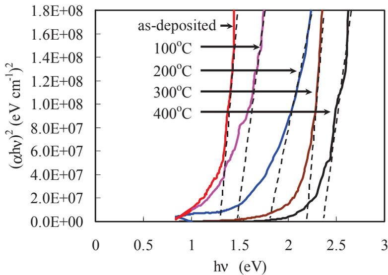
**Fig. 4.15. Bandgap estimation of the as-deposited film and the films annealed at the different temperatures.**
