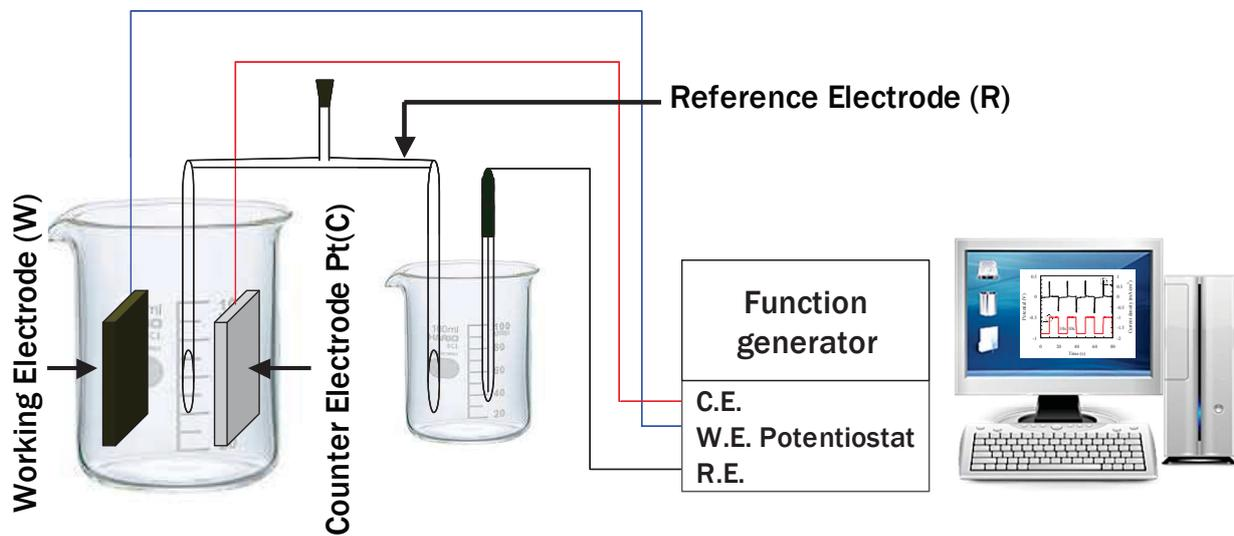
**Fig. 1.3. Schematic diagram of the 3-electrode cell apparatus used for electrochemical deposition of thin films.**
