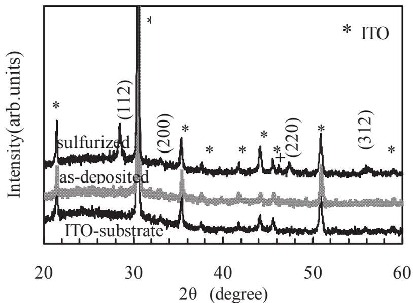
Fig. 3.18. XRD patterns of the as-deposited and sulfurized films on the ITO substrate.
