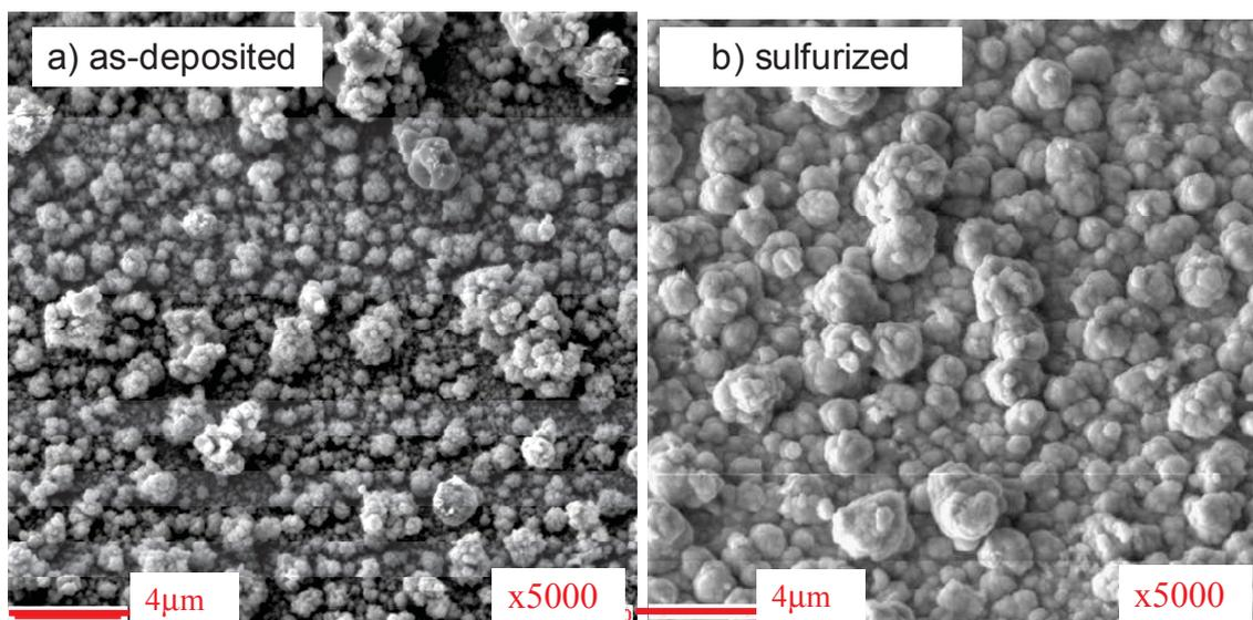
**Fig. 3.15. SEM image of the surface of the as-deposited and sulfurized film.**
