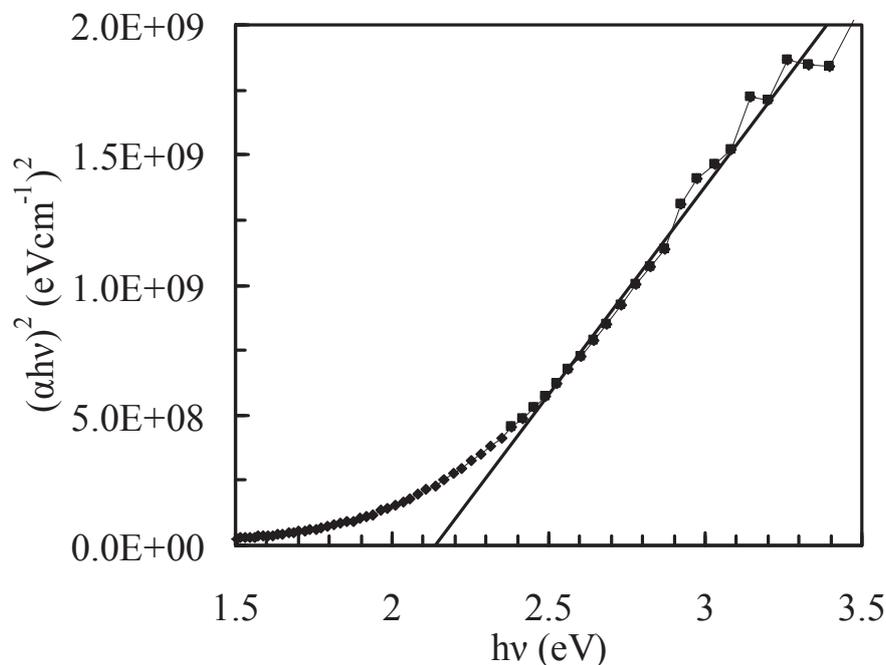
Fig. 2.6. Estimation of the band gap for the  $\text{Cu}_x\text{S}$  thin film.
