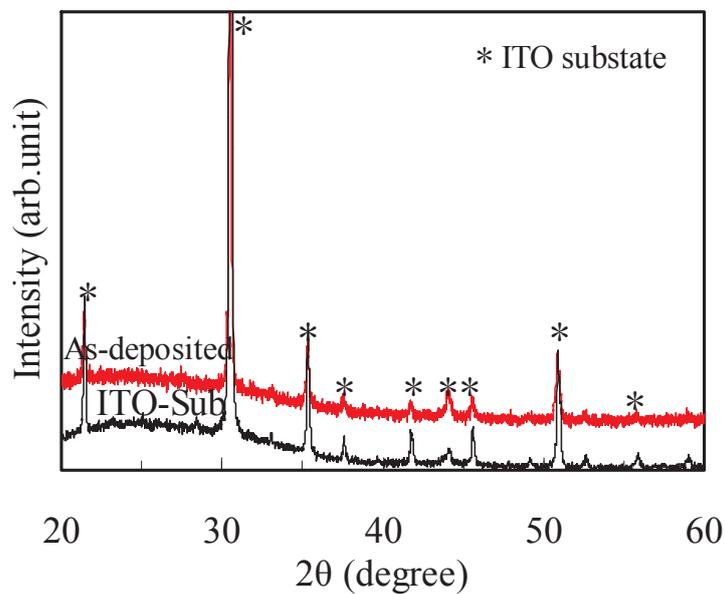
Fig. 4.9. X-ray diffraction pattern of the  $\text{FeS}_x\text{O}_y$  film on the ITO substrate.
