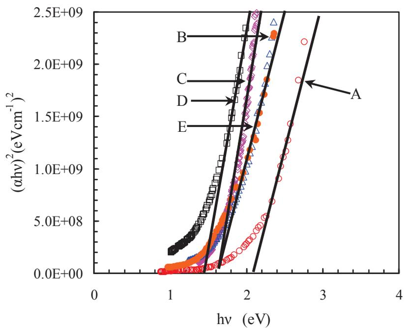
Fig. 3.7. Estimation of the band gap of the CZTSO samples (A, B, C, D, E).
