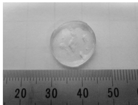
Fig.4-21 Photograph of 50P6F30-1.0 immersed in Toluene for 24hrs.
