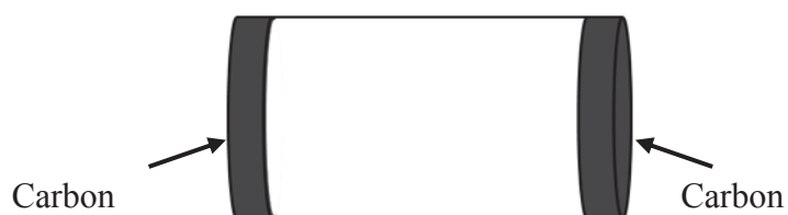
Fig. 2-5 Specimen used for impedance measurement.
