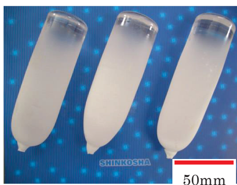
Fig. 2-2 Photograph of sapphire boules grown by FFM.
