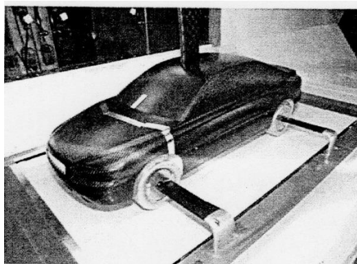
Fig. 1.11 Wind tunnel setup with 30% model (Lasse 2010 (11) ).
