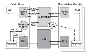
Fig. 3. Structure of a parallel speculative execution.
