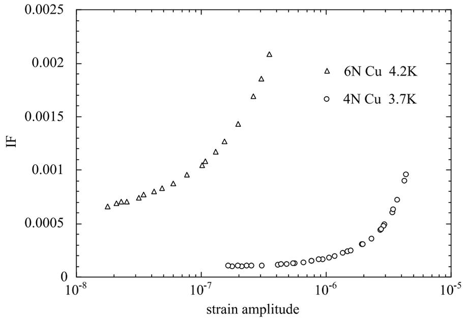
Fig. 4. Internal friction vs. strain amplitude in Cu crystals at 4 K.
