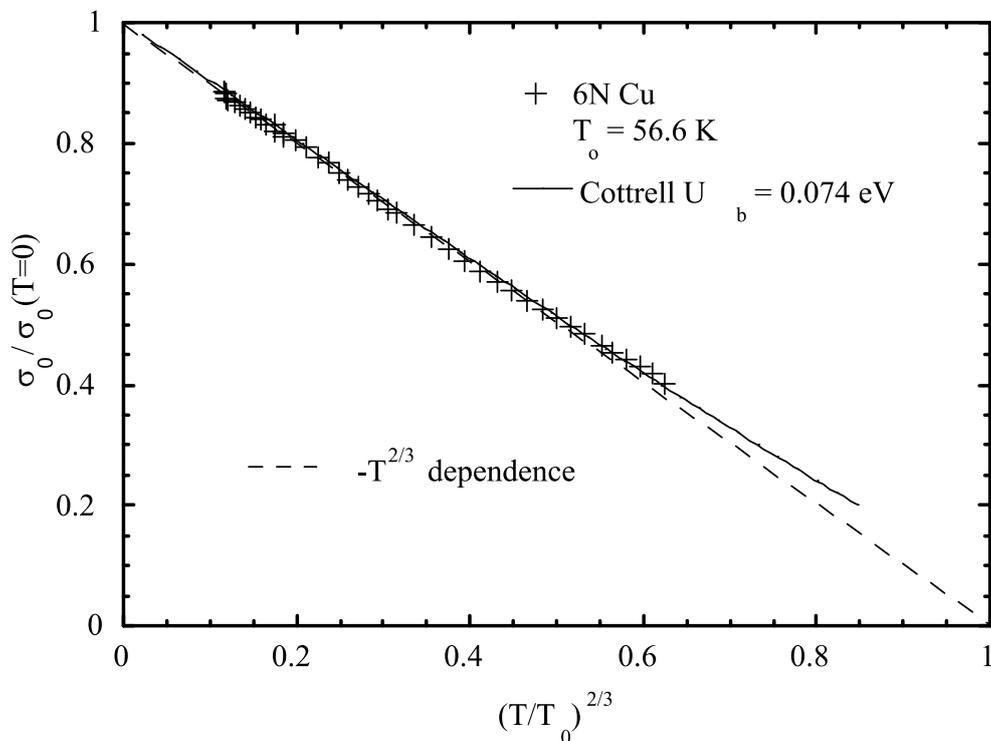
Fig. 5. The temperature dependence of the stress amplitude in 6N Cu necessary to produce a constant ADIF. The stress amplitude and temperature are normalized by extrapolated values of  $T^{2/3}$  dependence at low temperature.
