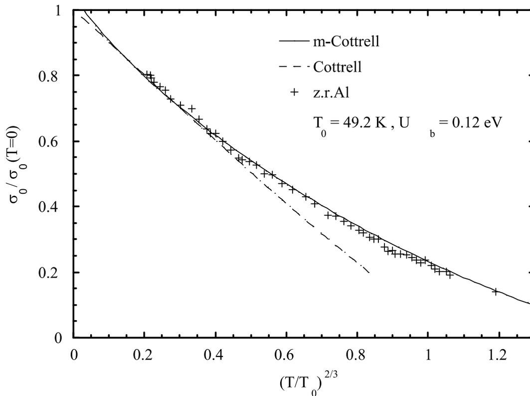
Fig. 3. The temperature dependence of stress amplitude in zone refined aluminum for producing the constant ADIF. The stress amplitude and temperature are normalized by extrapolated values of  $T^{2/3}$  dependence at lower temperature.
