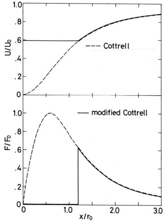
Fig. 2. Cottrell type potential  $U$  and force  $F$  (broken line) profile and a modified Cottrell potential profile (real line) vs. the distance between a dislocation and pinning atom. (right)
