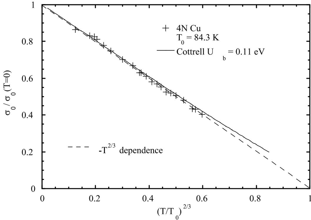
Fig. 6. The temperature dependence of stress amplitude in 4N Cu for producing the constant ADIF. The stress amplitude and temperature are normalized by extrapolated values of  $T^{2/3}$  dependence at low temperature.
