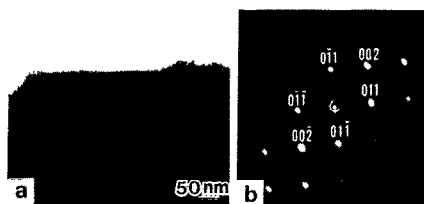
FIG. 11. TEM image of a Mo bulk target bombarded with 3-keV \text{N}_2^+ ions for 6 h. (a) Bright-field image and (b) corresponding ED pattern, showing the (100) reflection from the Mo lattice.
