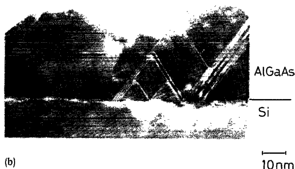
FIG. 2. (a) Conventional and (b) high-resolution TEM micrographs of \text{Al}_{0.5}\text{Ga}_{0.5}\text{As} on Si grown at 750^\circ\text{C} . The AlGaAs thickness is 22.5 nm.
