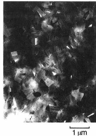
Fig. 5. TEM photograph of the glass-ceramic containing 6 wt% \text{Ca}_3(\text{PO}_4)_2 in BCTM system.
