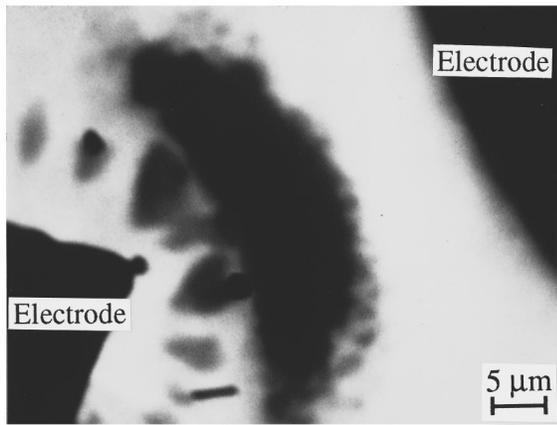
FIG. 4. EBIC image of degraded InGaN/AlGaIn LED shown in Fig. 3(c).
