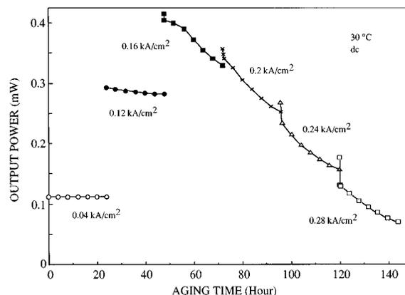
FIG. 1. Variation of output power from InGaN/AlGaIn LED as a function of aging time under various injected current densities. Each aging test was performed for 24 h at  $30^\circ\text{C}$ .
