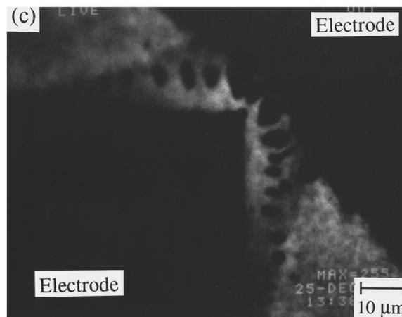
FIG. 3. EL images of progressive stages of degradation for InGaN/AlGaIn LED during the aging test under 0.4 kA/cm<sup>2</sup> at 30 °C, (a), (b), and (c) correspond to initial stage and aging of 67 and 310 h, respectively.
