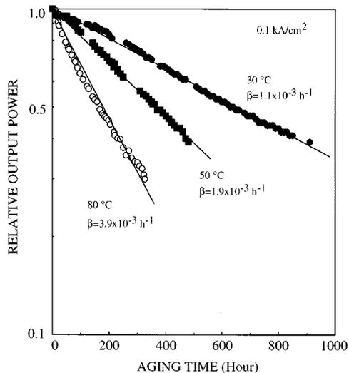
FIG. 2. Variation of relative output power from InGaN/AlGaIn LED as a function of aging time at ambient temperatures of 30, 50, and 80 °C. The injected current density was 0.1 kA/cm<sup>2</sup>.
