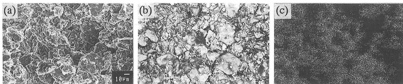
Fig. 2. SEM photographs of fracture surfaces of C/SiO 2 composites with 4.6 vol% graphite: (a) SE image, (b) BE image and (c) Si mapping.
