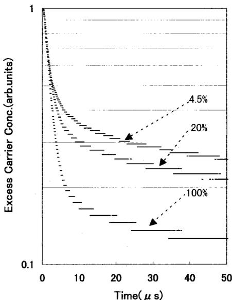
FIG. 3. Excess carrier decay curves of 3C-SiC/Si for various excitation strengths. The  $N_2$  laser is used for excitation, and the intensity on the sample surface was varied from 100% to 4.5% of the initial output using filters.
