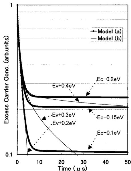
FIG. 6. Calculated decay curves for various values of the trap level. The model Fig. 4(a) is assumed for the bold lines and the model Fig. 4(b) for the thin lines.  $\sigma_n$  is  $1 \times 10^{-22} \text{ cm}^2$  and  $n_d$   $5 \times 10^{15} \text{ cm}^{-3}$ .
