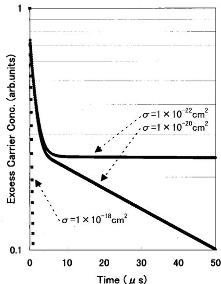
FIG. 5. Decay curves calculated with the electron capture cross section of the trap  $\sigma_n$  as a parameter. The trap level and concentration are 1.0 eV and  $5 \times 10^{15} \text{ cm}^{-3}$ , respectively.
