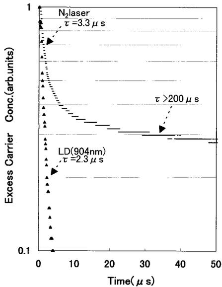
FIG. 2. Decay curves of excess carrier concentration in 3C-SiC/Si measured by the  $\mu$ -PCD method. The decay curve has a single time constant when the laser diode was used for excitation, while it has a fast component ( $\tau \approx 3 \mu\text{s}$ ) and a slow one ( $\tau > 200 \mu\text{s}$ ) under the  $N_2$  laser excitation.
