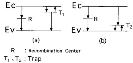
FIG. 4. Two defect models assumed in the simulation of the excess carrier decay curves.
