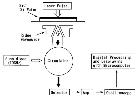
FIG. 1. Schematic illustration of apparatus for the  $\mu$ -PCD measurement.
