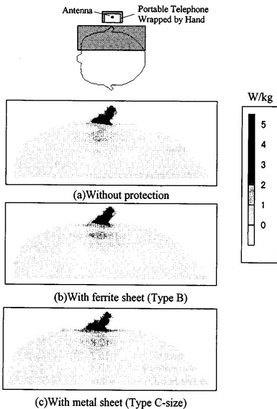
Fig. 5 SAR distributions in a horizontal cross section through the center of eyes. Only the shadow area is shown.
