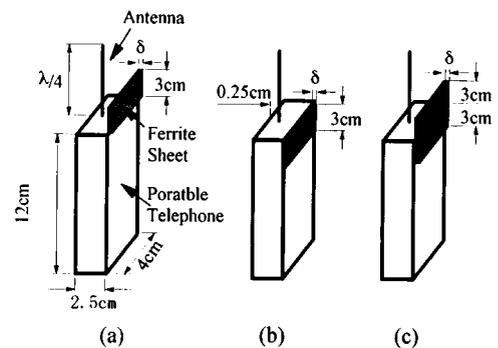
Fig. 2 Portable telephones with ferrite sheets. (a) Type A, (b) Type B, (c) Type C.
