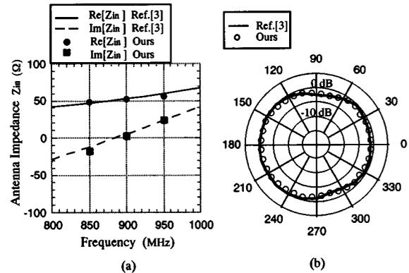
Fig. 4 Test results of our FDTD code. (a) Antenna impedance, (b) Radiation pattern in  $\phi$ -plane.
