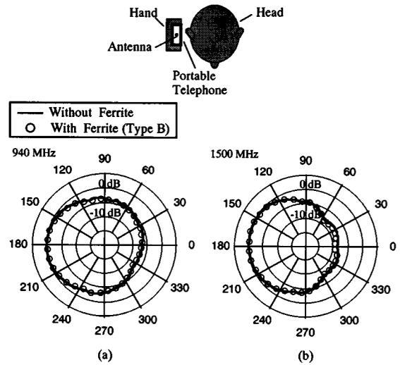
Fig. 6 Radiation patterns in  $\phi$ -plane for a monopole antenna on a dielectric covered metal box for the anatomically based head model. (a) 940 MHz, (b) 1500 MHz.
