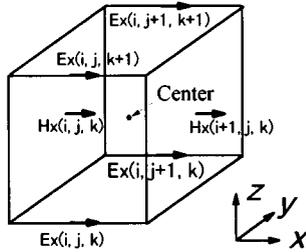
Fig. 3 View of calculation for  $E$  and  $H$  in the center of the cell.
