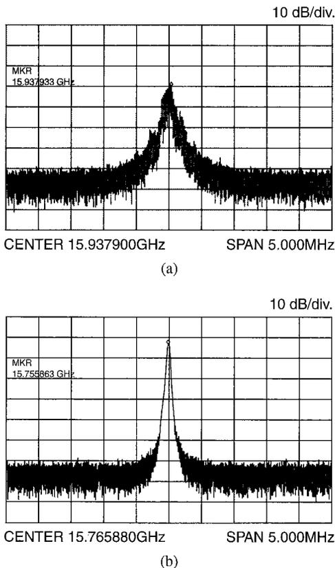
Fig. 4 Measured frequency spectra for the oscillators with (a) one HEMT and (b) nine HEMT's.
