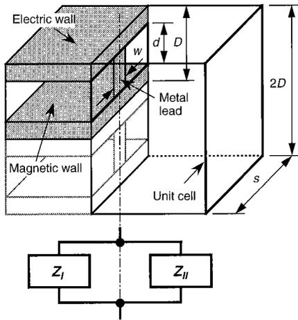
Fig. A · 1 Calculation model for the lead impedance in the unit cell.
