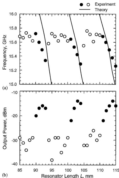
**Fig. 6** (a) Measured oscillation frequencies and (b) output power for the oscillator with one HEMT, as a function of the resonator length. The solid lines in (a) indicate the theoretically calculated frequencies.
