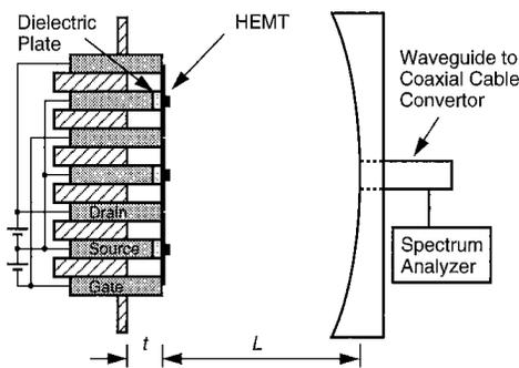
Fig. 3 Experimental setup at Ku-band.
