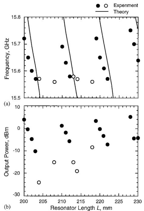
Fig. 5 (a) Measured oscillation frequencies and (b) output power for the oscillator with nine HEMT's, as a function of the resonator length. The solid lines in (a) indicate the theoretically calculated frequencies.
