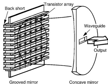
Fig. 1 A grooved-mirror type quasi-optical oscillator.
