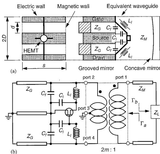
Fig. 2 (a) The unit cell and (b) the equivalent circuit for the HEMT array in the resonator.
