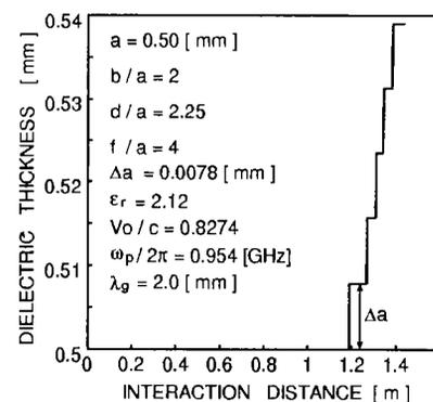
Fig. 2 Spatial variation of the dielectric thickness.  $V_0$  refers to the initial velocity of the electron beam,  $\epsilon_r$  the relative permittivity of dielectric,  $\omega_p$  the plasma frequency of the electron beam,  $c$  the speed of light in vacuum, and  $\lambda_g$  the guide wavelength.
