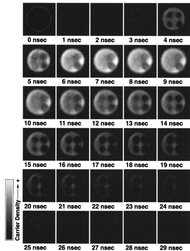
FIG. 2. Temporal evolution of photoexcited free carrier distribution. The image size is  $3220 \mu\text{m} \times 3220 \mu\text{m}$ . The time under each image indicates the time after the photoexcitation began. The time division is 1 ns.
