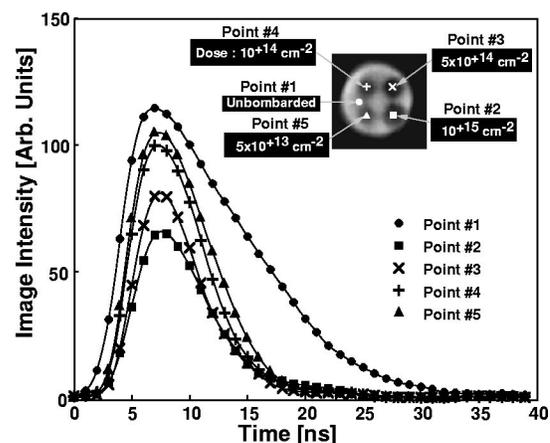
FIG. 3. Temporal changes of image intensities. Point 1 is the unbombarded region, and Points 2–5 are the ion bombarded regions with doses of  $5 \times 10^{13}$ ,  $10^{14}$ ,  $5 \times 10^{14}$ , and  $10^{15} \text{ cm}^{-2}$ , respectively.
