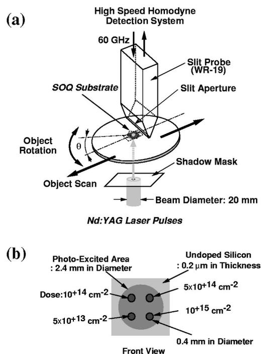
FIG. 1. Experimental scheme for visualizing transition phenomena of photoexcited free carriers in reflection mode: (a) experimental setup and (b) sample configuration. The experimental conditions in data acquisition are as follows: sampling interval for linear scan is  $60 \mu\text{m}$ , sampling points for linear scan, 74 points, sampling interval for rotational scan,  $2.43^\circ$ , total number of linear scans, 74, and probe-to-object separation,  $10 \mu\text{m}$ .
